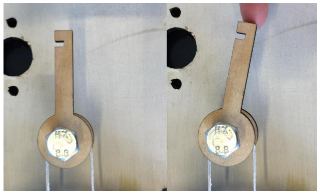
Figure 16-2: Slack shown on thumb joint.
