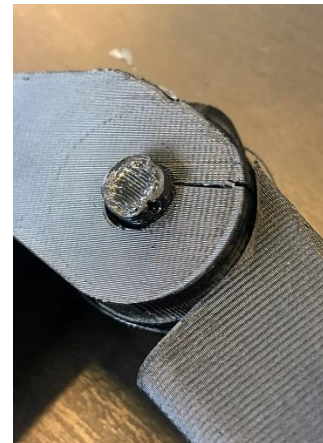
Figure 12-3: A bearing encasement broke because the mechanical tolerances were too small.
