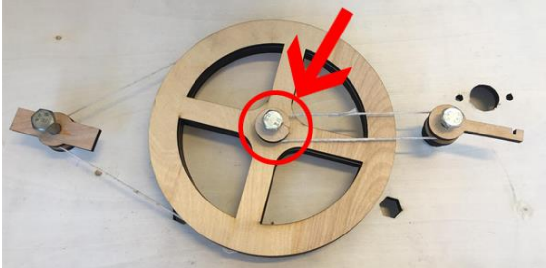
Figure 16-3: Slippage occurred here.
