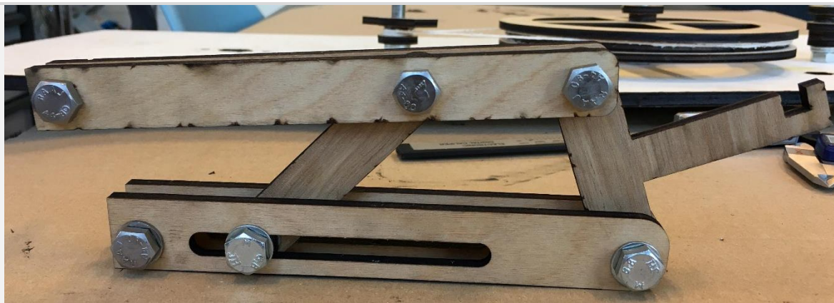
Figure 6-3: Prototype for linkages using design from adjustable lock pliers.
