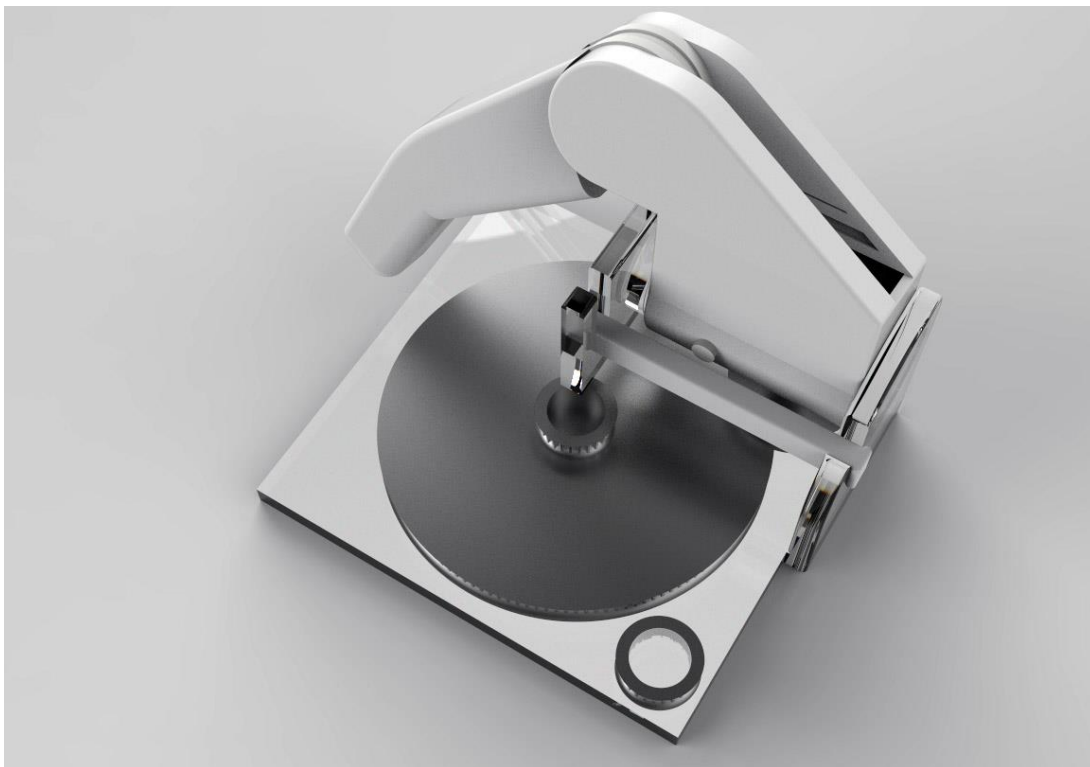
Figure 11-2: Render showing the assembled thumb and base (in acrylic) prototype from above.
