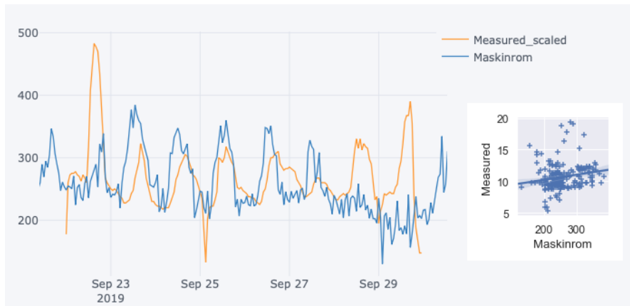
Figure 4.6: Plots of hourly values of machine room consumption and nearby outside temperatures (which is upscaled by factor 25), from Sept 22nd till Sept 29th. A corresponding correlation plot is found on the right.
