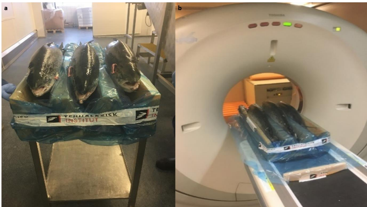
Figure 3.1 (a) Fish set on prepared fixture ready for CT scanner and (b) Scanning of fish.
