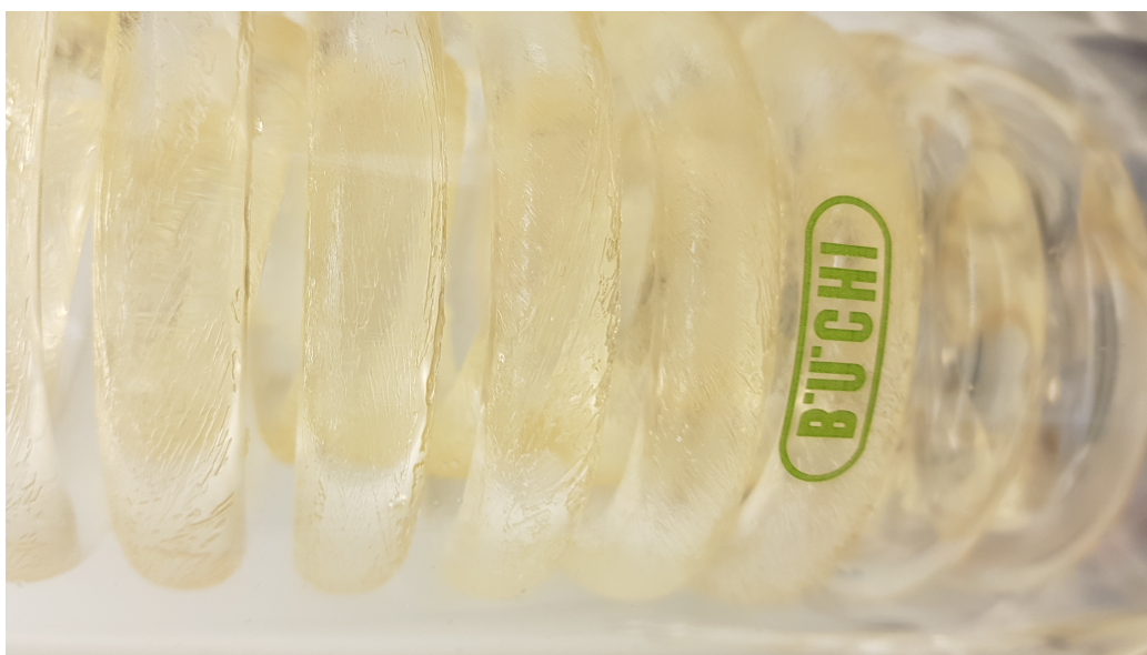
Figure 5.3: Picture of icing of t-BuOH in the cooling column inside the rotary evaporator
