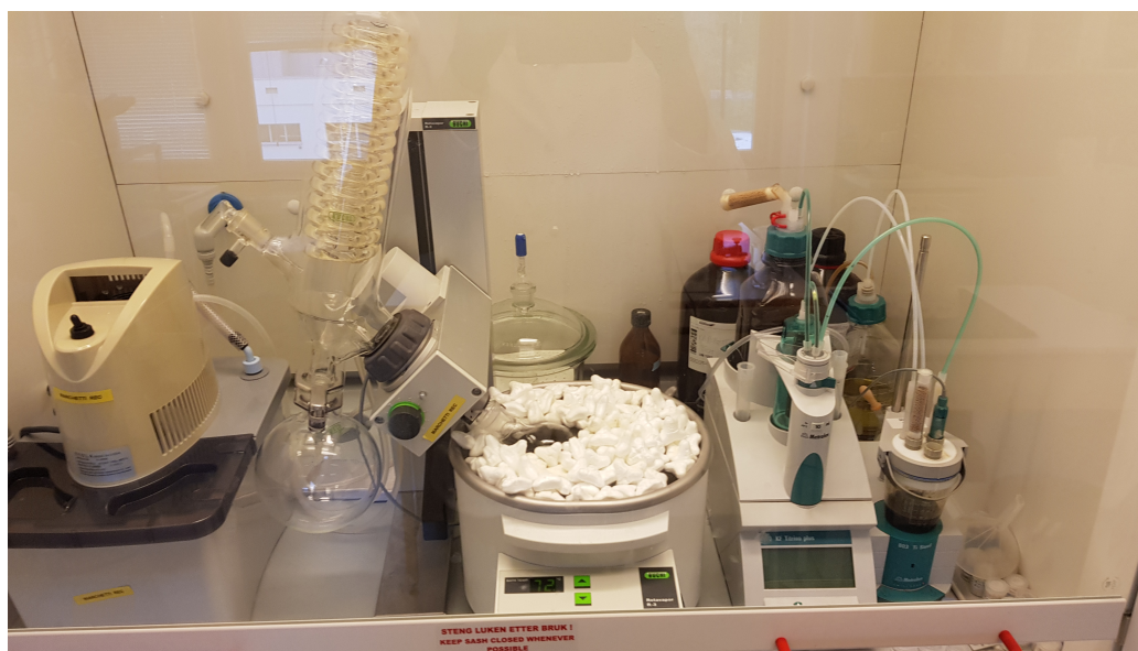
Figure 3.4: Picture of the Rotavapor R-3 , with the vacuum pump to the left.
