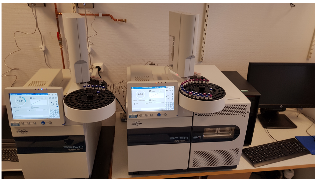
Figure 3.3: Picture of GC setup, GC to the left and GC-MS to the right.
