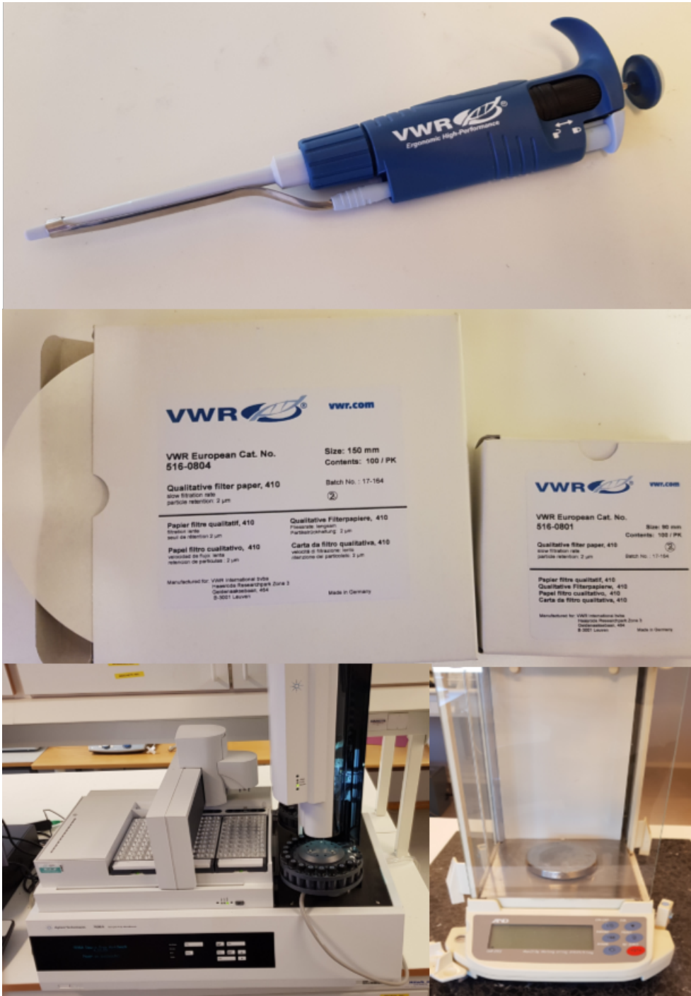
Figure 3.5: Pictures of some equipment used. \mu -pipette at the top, filter papers below, prep-bench at the bottom left and the scale in the bottom right.
