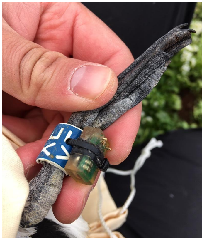
Figure 3: Geolocator of type Mk4083 (Biotrack) mounted on to the plastic identification ring wrapped around the leg of a razorbill. Photo: Magne Hestem
