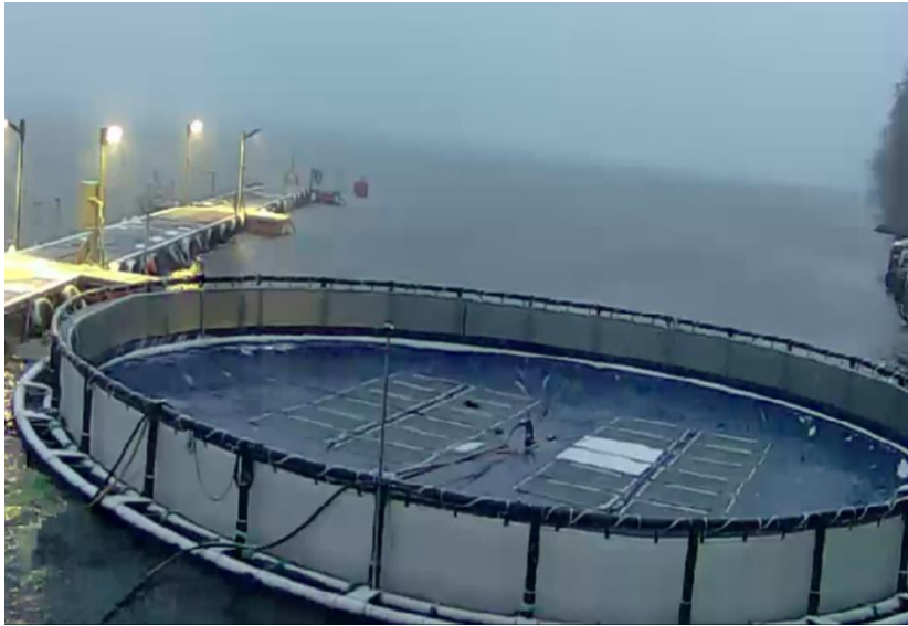
Figure 20: Picture of the system 08:30 the day after the modules were lifted. The two white modules are the ones that were lifted and display signs of frost on their surface.
