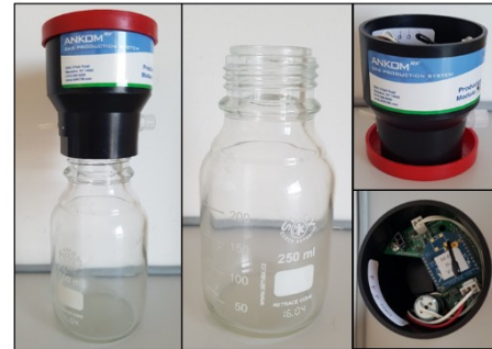
Figure 4. Bottles and heads containing pressure sensor modules for the ANKOM Gas production system. The knob on the right side of the head is an automated valve to realise gas during incubation.
