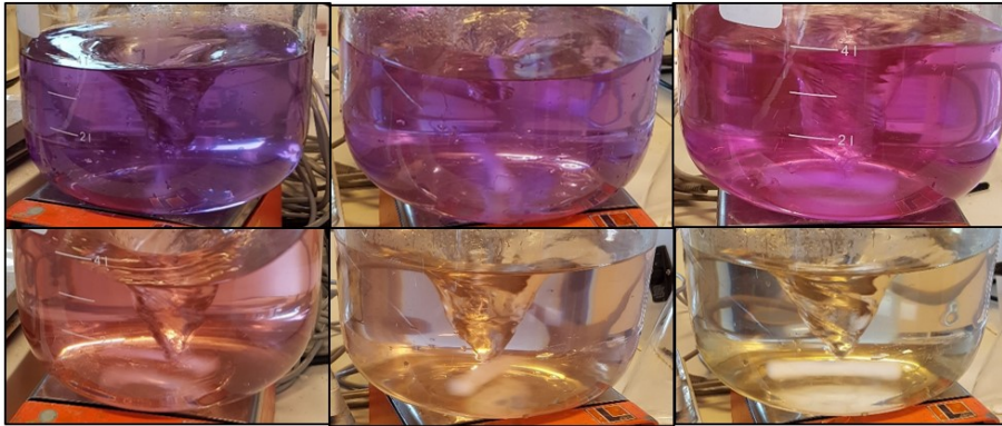
Figure 8. The colour change in the buffer solution from the original blue/purple to transparent. This takes approximately 30 minutes.
