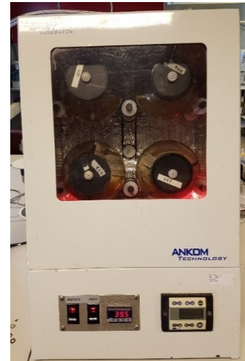
Figure 3. A picture of the ANKOM Daisy II Incubator during incubation.
