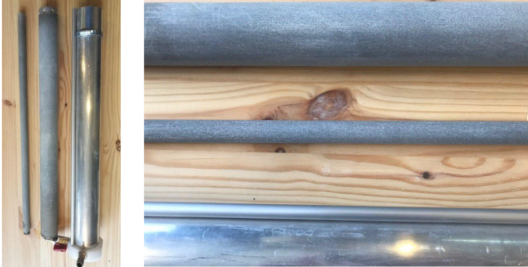
Figure 39. Appearance of electrodes after all the tests
