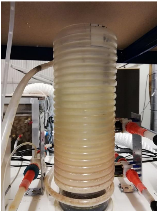
Figure A2. Flocculating tubes
