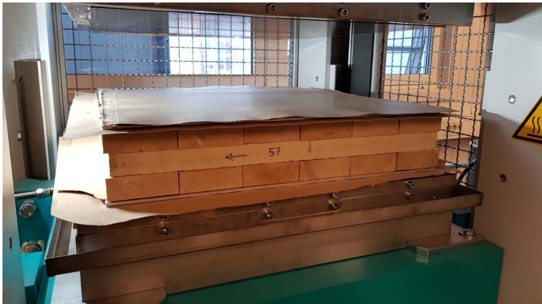
Figure 20: Manufacturing of composite CLT panel at NIBIO
