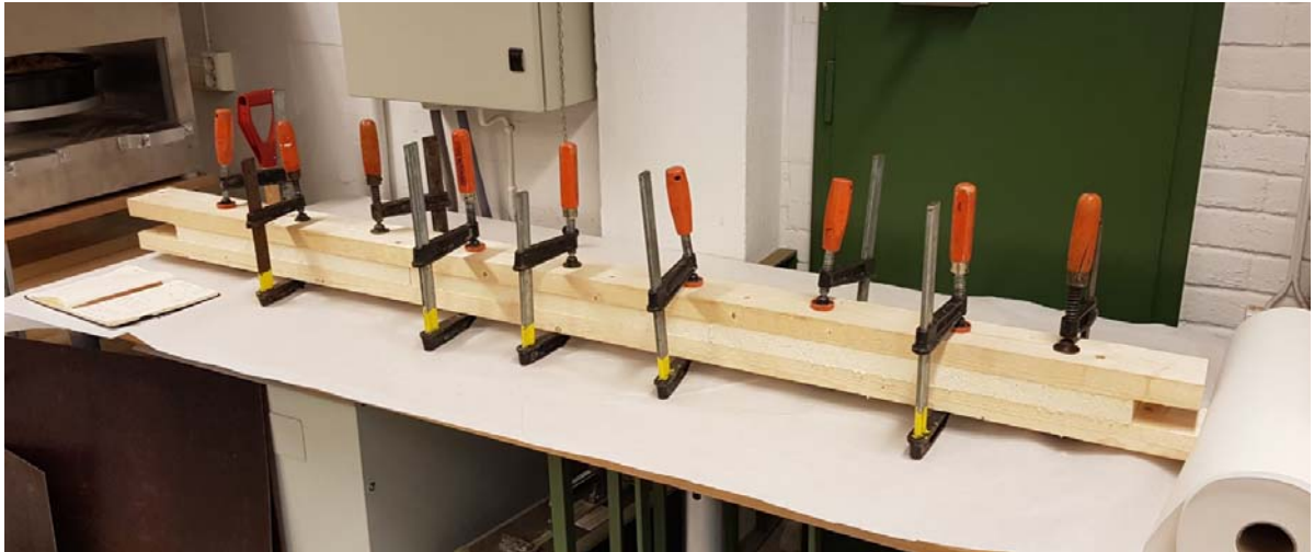
Figure 29: Assembly of the bending test specimen
