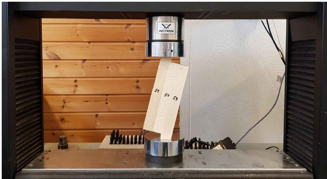
Figure 24: Experimental setup for shear tests
