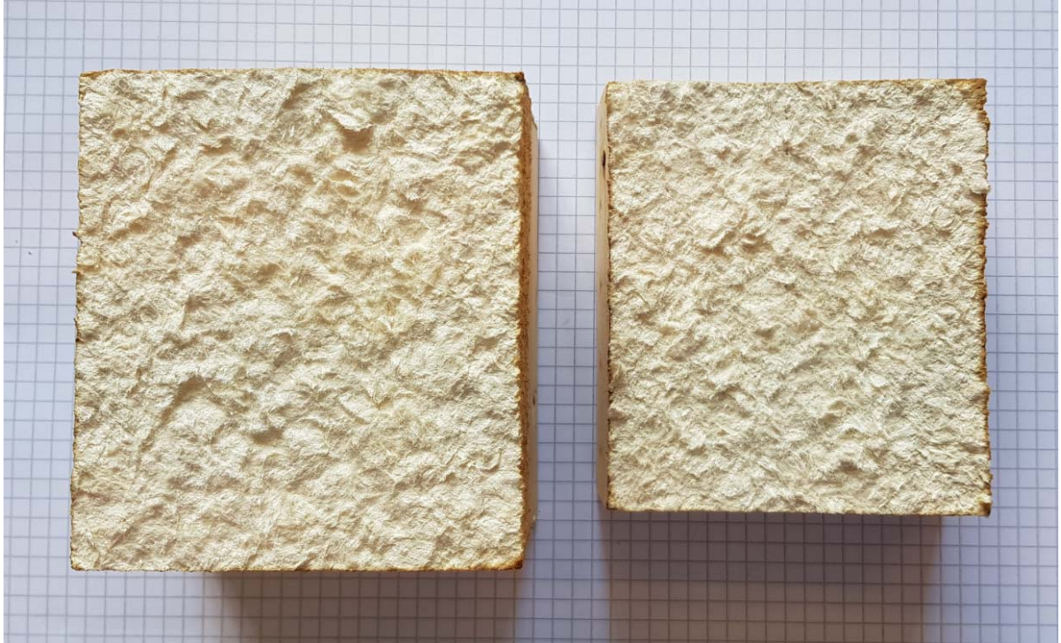
Figure 44: Typical mode of failure for delamination tests
