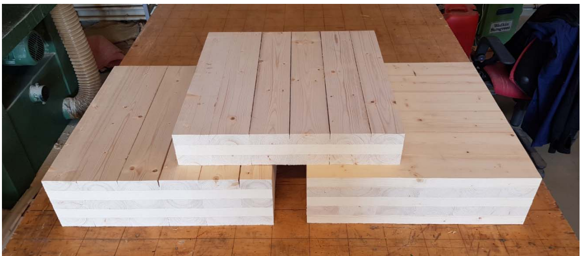
Figure 33: In-plane test samples upon completion
