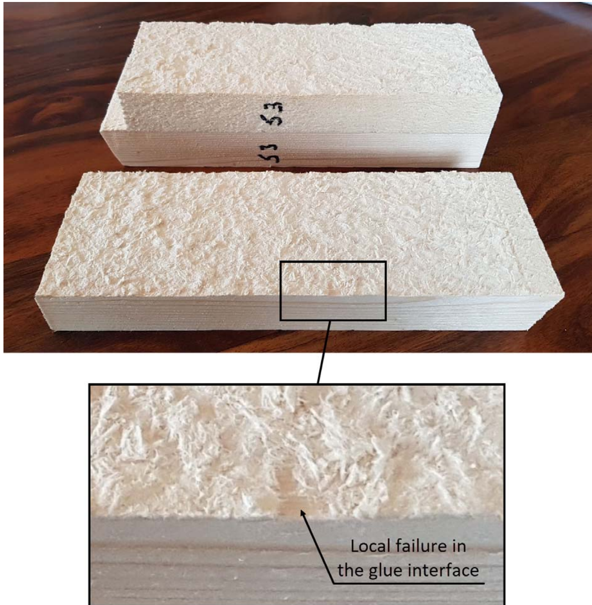
Figure 37: Typical mode of failure for shear tests
