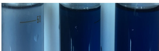
Figure 12 – Ozone determination by Indigo method
