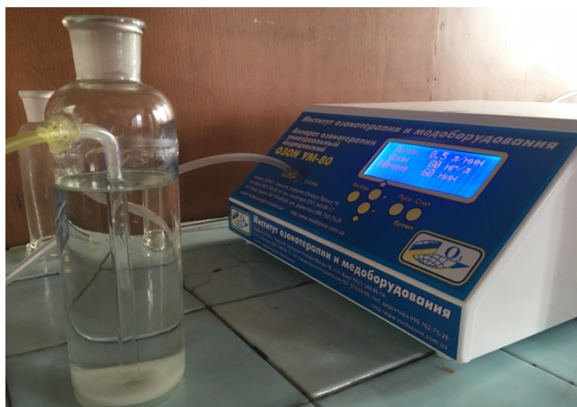
Figure 11 - The Ozonation set-up
