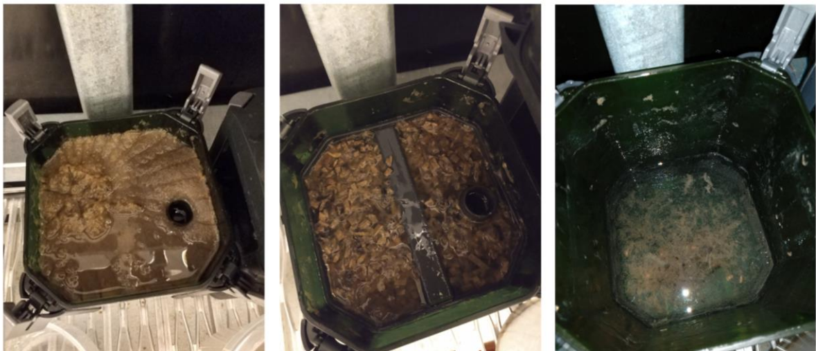
Figure 4.17: Visual inspections of the units after finishing the experiment. Clear accumulation of organic material in the reactors and signs of decomposing of the woodchip media.
