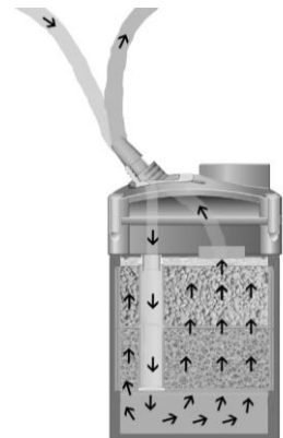
Figure 3.5: Flow in the filtration systems (Eheim GmbH & CO. KG, 2019) (modified).
