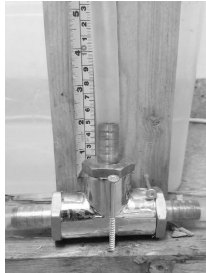
Figure 3.13: T-connection connecting the water column hose to the system.
