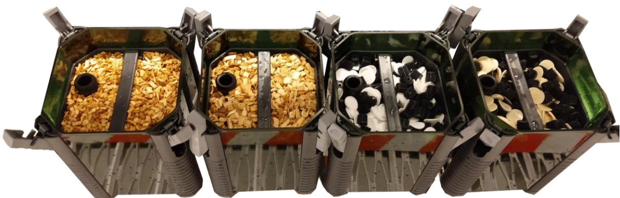
Figure 3.3: The four different media used in the experiment; Small woodchips, big woodchips, new plastic and already cultured plastic media.
