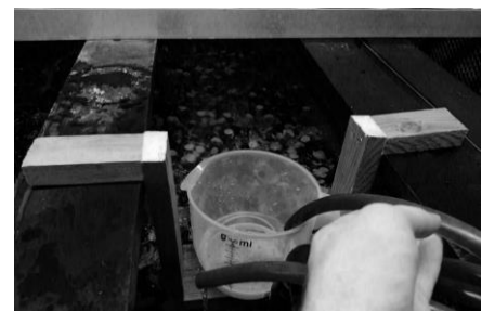
Figure 3.7: Setup for measuring flowrate of the filtration units.
