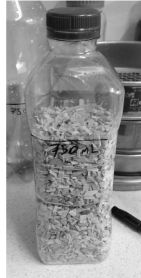
Figure 3.10: Porosity experiment set up. Bottle with volume marking, filled with media and water to determine void volume.
