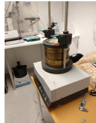
Figure 3.2: A Retch AS 200 control laboratory sieve shaker were used to separate the particles in different sizes.
