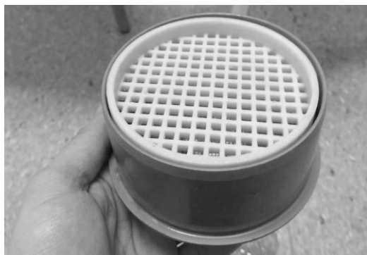
Figure 3.14: Flow break-up device. Designed in Solidworks Flow Simulation and 3D-printed.
