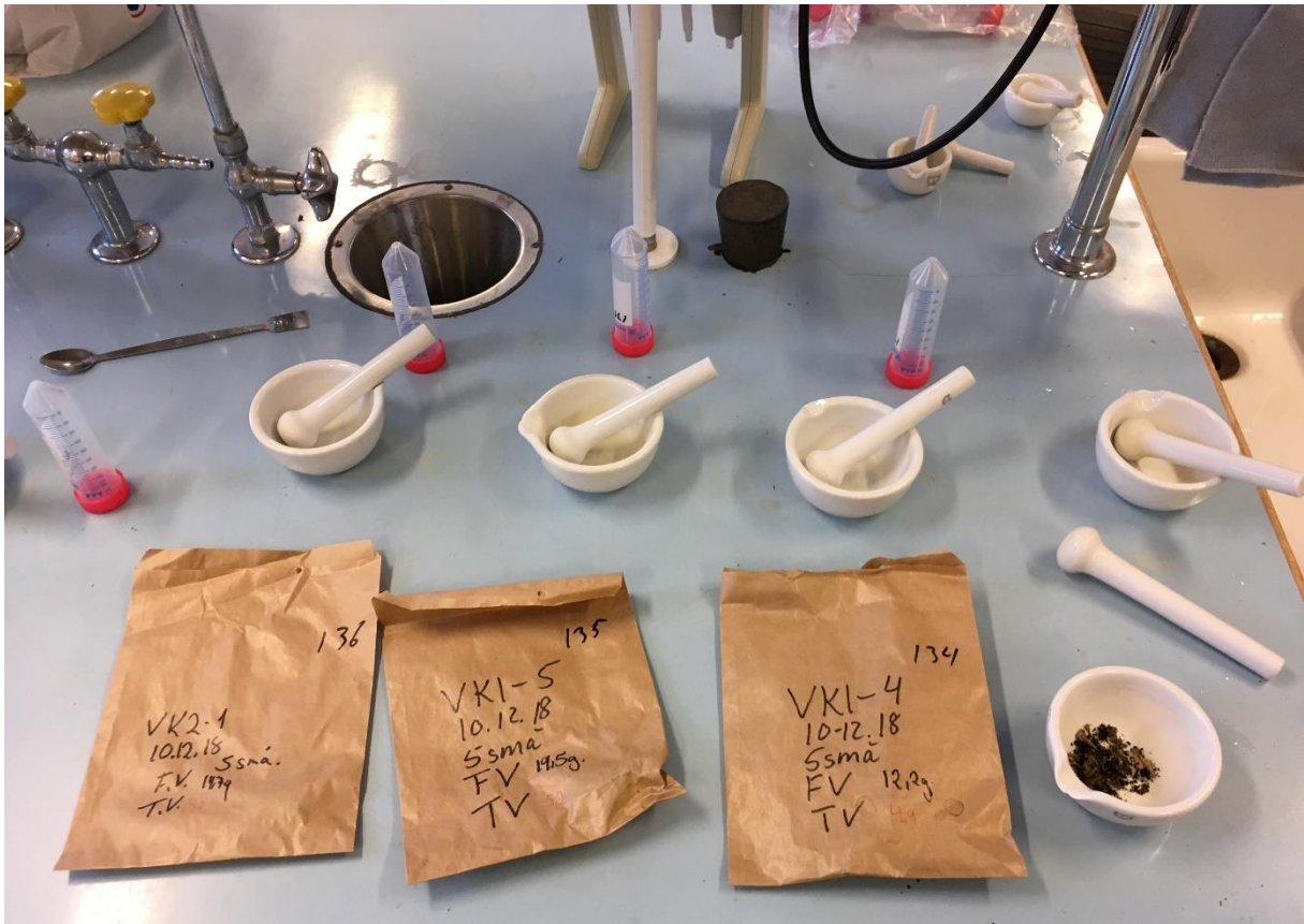
Figure 31: The mortars with cylinders for each sample lined up with the sample bags in the front. Photo: Martin Knoop.
