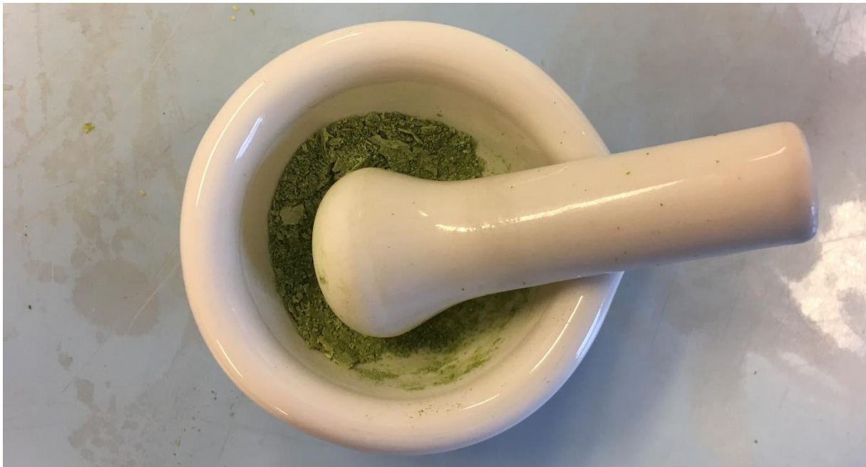
Figure 32: Showing a mortar with a sample ground halfway to powder. Photo: Martin Knoop.
