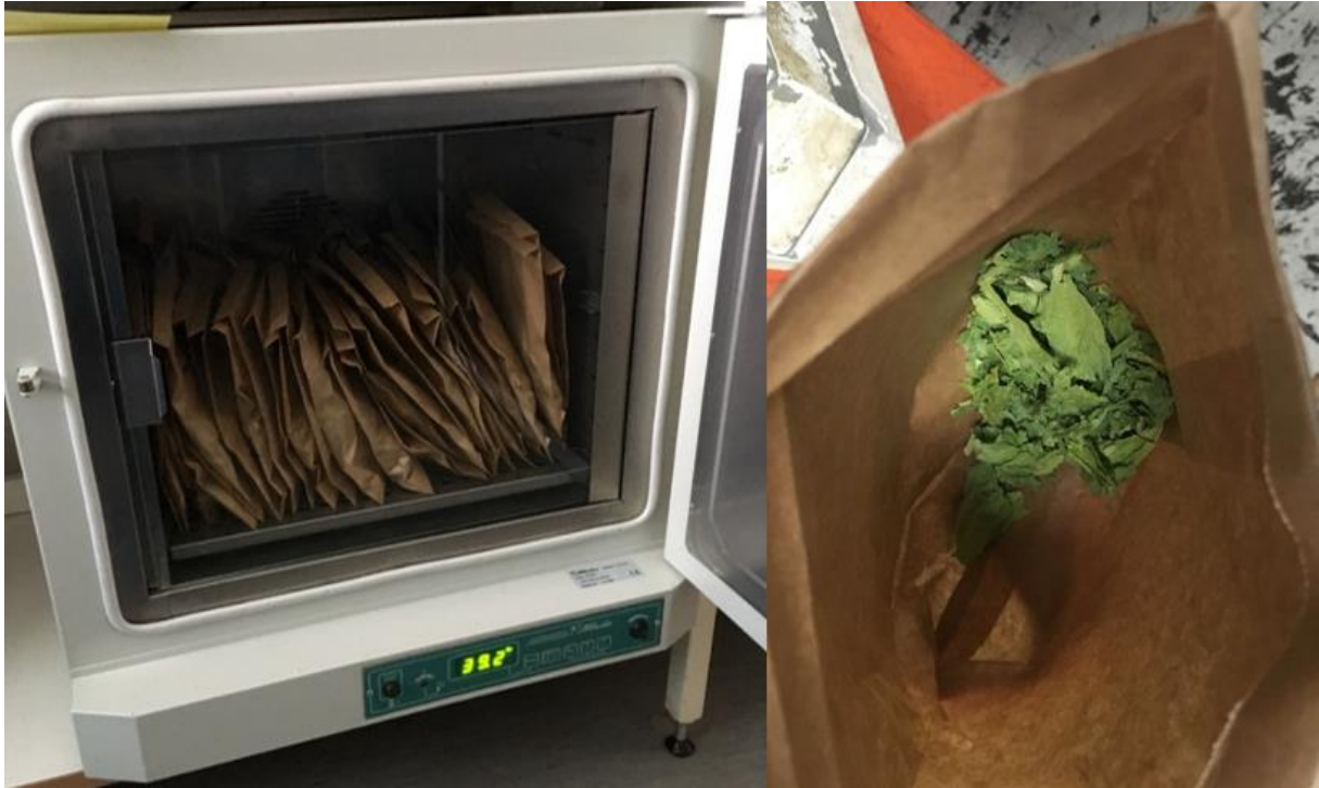
Figure 29: Heating oven warming up to 45°Celsius with the samples inside. Figure 29.1: Dried samples crushed inside the bag for further processing. Photo: Martin Knoop.
