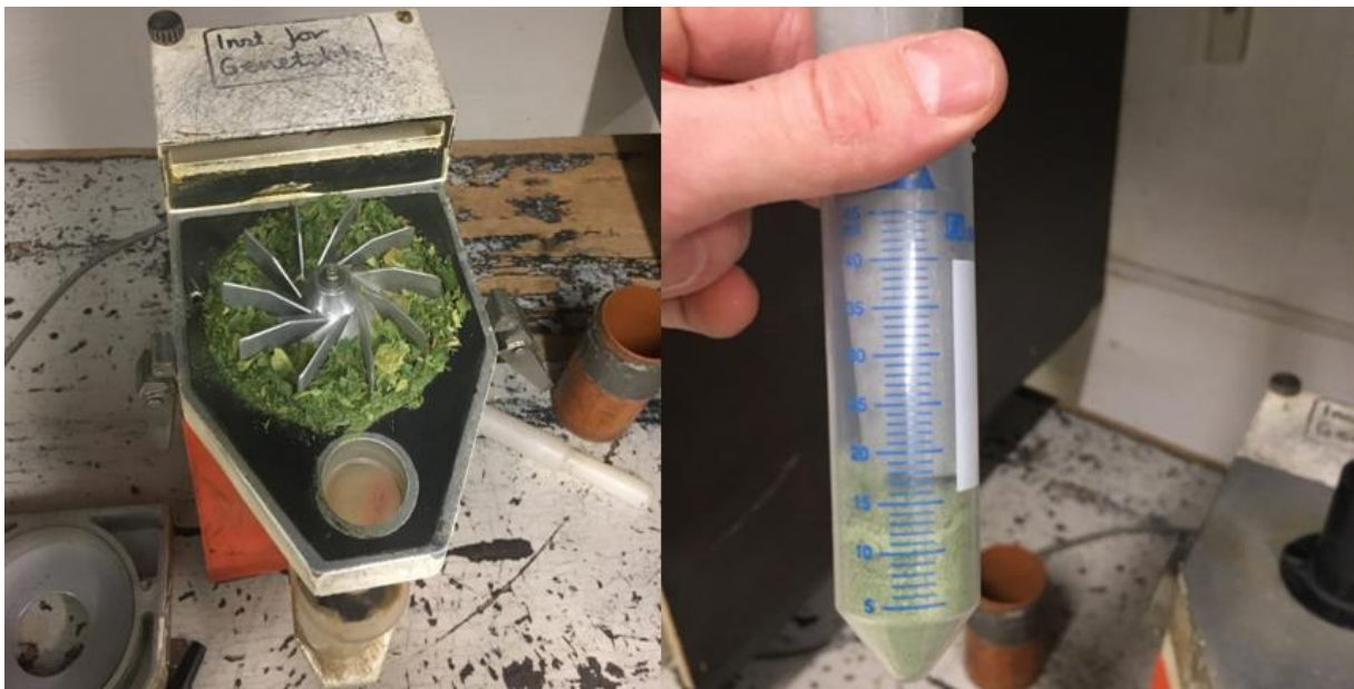
Figure 30: Grinder with the lid off (in the left corner) chopping up the salad and putting it into the container glass (in the middle bottom of the picture). Figure 30.1: Cylinder containing a sample prepared to be sent off to the lab. Photo: Martin Knoop.
