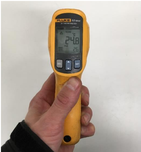
Figure 27: Infrared sensor for measuring leaf temperature. Photo: Martin Knoop.
