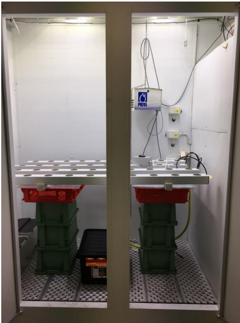
Figure 10: Showing growth chamber 1 with the black plastic box between the pillars the gutters rest on, and the yellow hose bringing water up to the black hoses to the right connected to the 4 gutters. To the left the water leaves the gutters and enters the transparent plastic boxes below. On top of the gutters lies the timer that starts the water pump every other hour. (The timer was hanging from the S-hook up in the right-hand corner). Photo: Martin Knoop.
