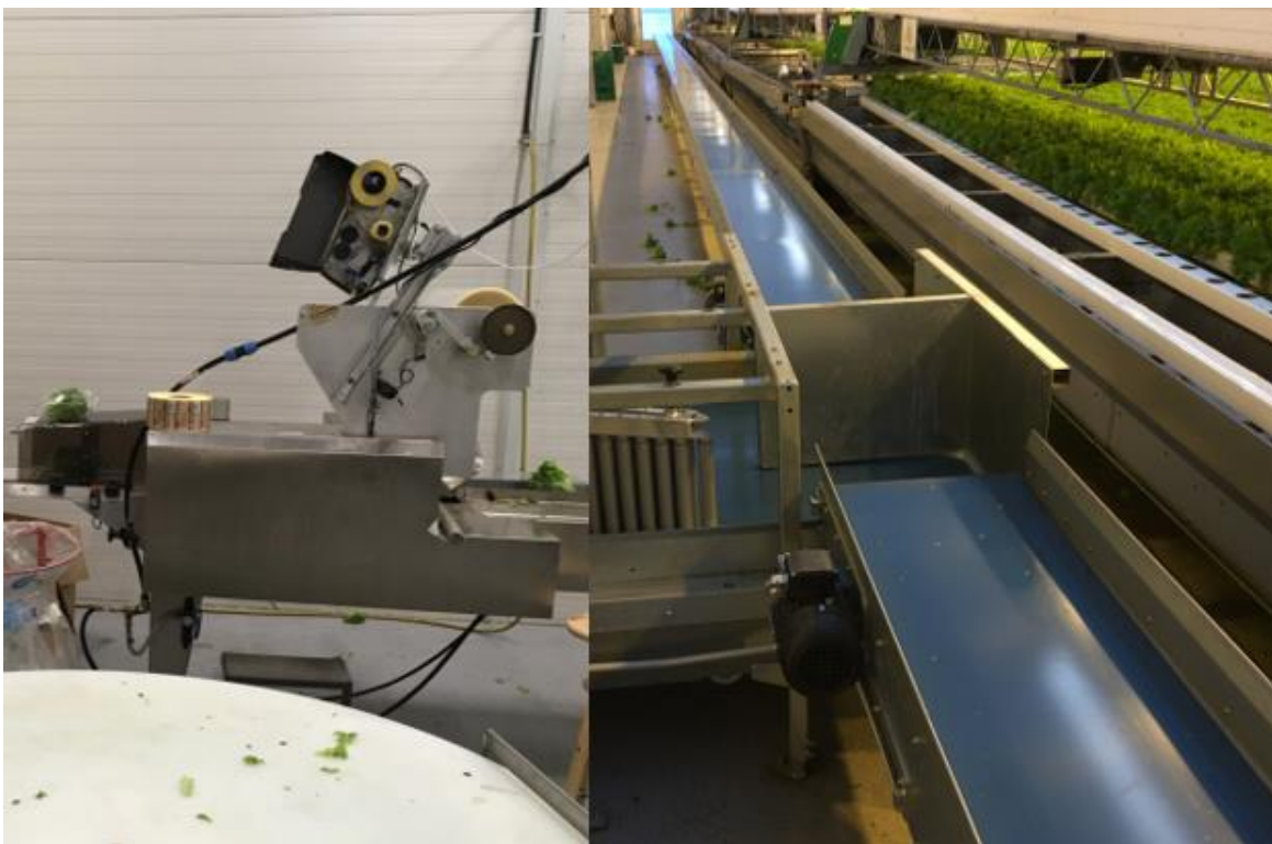
Figure 4: Harvest-ready lettuce (to the right) is cut and put onto the conveyor belt, and packed in plastic (to the left). Picture taken at O Espedal Handelsgartneri. Photo: Martin Knoop.
