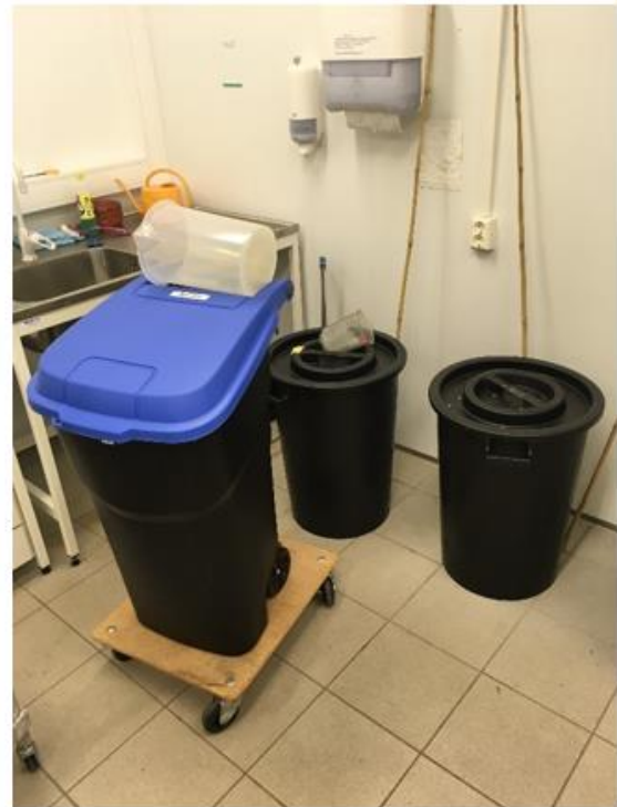
Figure 14: EC-meter used to measure the EC of the final fertilizer solution. Figure 14.1: The two stock solutions tanks seen in the back and the bigger tank with the final solution (with blue lid) standing on wheels so it's easier to move. The black troughs had to be refilled maybe 2 times a week from this tank. Photos: Martin Knoop.
