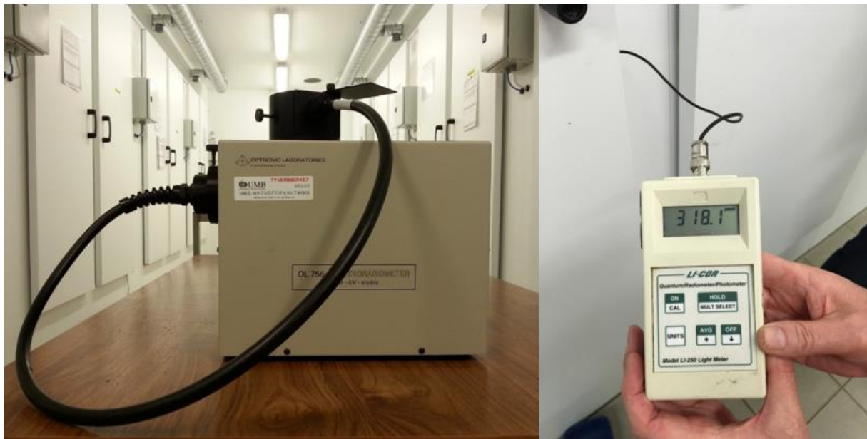
Figure 16: Optronic model 756 spectroradiometer used for measuring spectral composition of the different lighting. Figure 13.2: A quantum-meter was used to measure the achieved light intensity/photon flux. In this instance the lighting was 318 \mu\text{mol m}^{-2} \text{s}^{-1} . The goal in this case was 300 \mu\text{mol m}^{-2} \text{s}^{-1} \pm 10\% . Photo: Martin Knoop.
