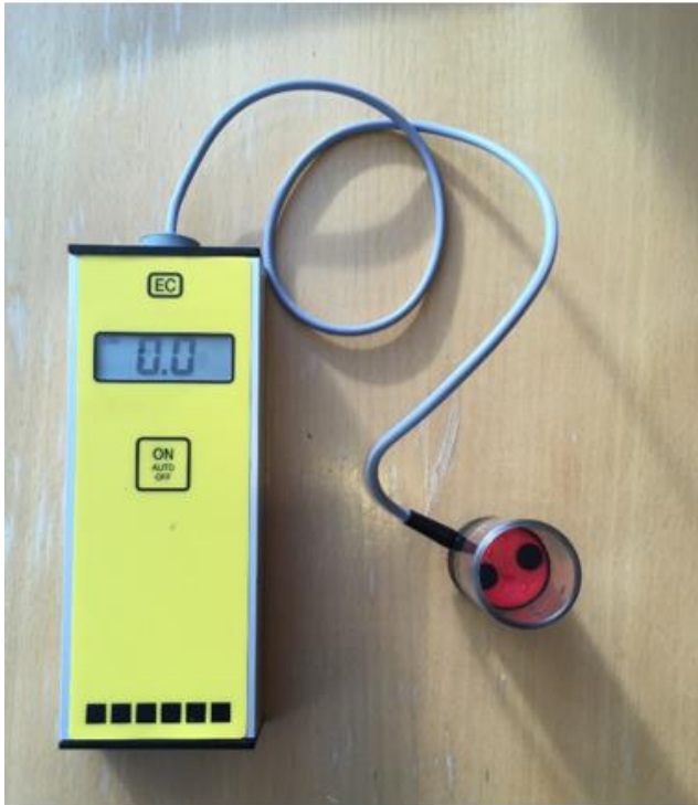
Figure 14: EC-meter used to measure the EC of the final fertilizer solution. Figure 14.1: The two stock solutions tanks seen in the back and the bigger tank with the final solution (with blue lid) standing on wheels so it's easier to move. The black troughs had to be refilled maybe 2 times a week from this tank. Photos: Martin Knoop.
