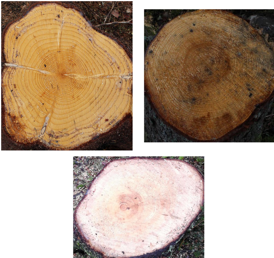
Figure 7.1: False positive classifications. All the images have areas of discolouration that could be RBR.
