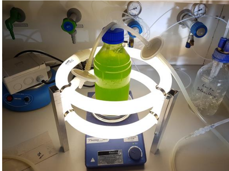
Figure 3: Preculture of Acutodesmus obliquus illuminated by a white light Sylvania light bulb and kept in motion by a magnetic stirrer and pressurised air mixed with CO 2 .
