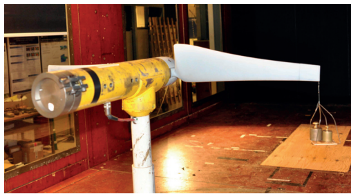
Figure 2.14: Calibration process of torque transducer.
