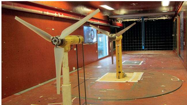
Figure 3: Turbine array with counter- rotating rotors in NTNUs wind tunnel at a separation distance of 3.5D
