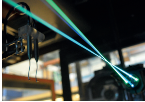
Figure 2.17: Simultaneous measurements with LDV and Cobra probe for adjustment of Cobra probe head.
