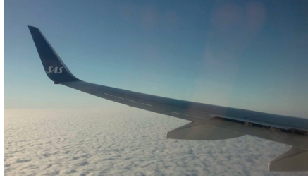
Figure 3.2: Winglet on the wing tip of a transport airplane.
