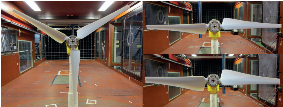
Figure 2.9: Model rotors for the experiment comparing the effect of the blade number on the wake development, mounted on model turbine T2 (taken from Paper I ).
