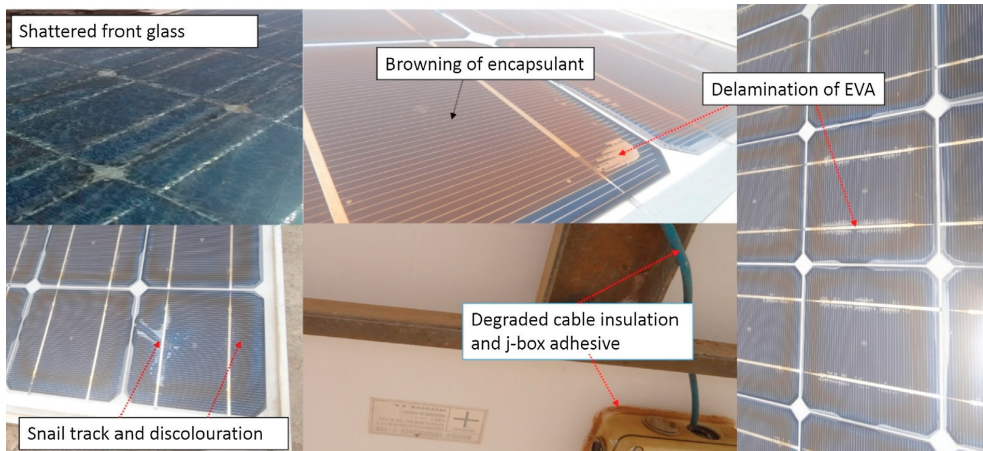
Fig. 13. Samples of observed defects in modules.
