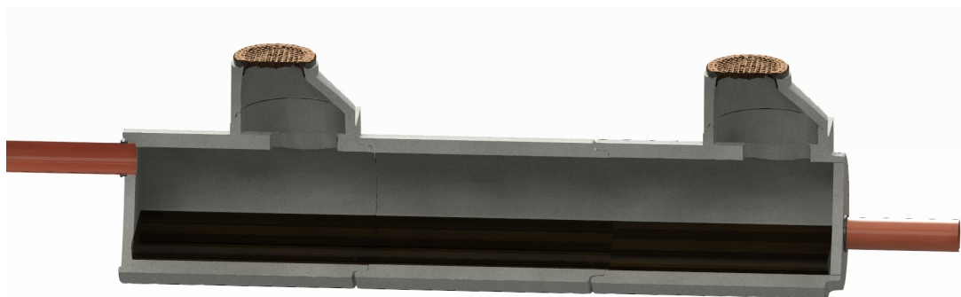
Figure 2.9: Cross section of a typical cylindrical sedimentation basin. Copied and illustrated by BASAL AS.
