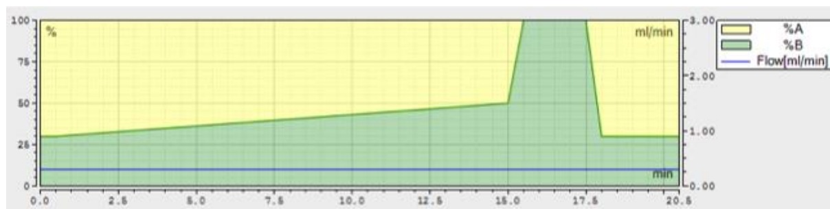
Figure B1: Mobile phase gradient profile 1, shown as a graph with percent on the y-axis and time on the x-axis.
