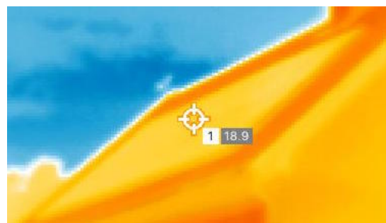
Figure C.9: Two thermal images of system 14, taken from different angles, indicating a constant temperature over the entire system. Note that the absolute temperatures shown in the images is wrong as temperature and emissivity references were not possible to set.
