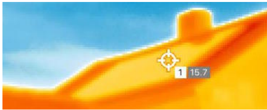
Figure C.5: Two thermal images of system 6, taken from different angles, indicating a constant temperature over the entire system. Note that the absolute temperatures shown in the images is wrong as temperature and emissivity references were not possible to set.
