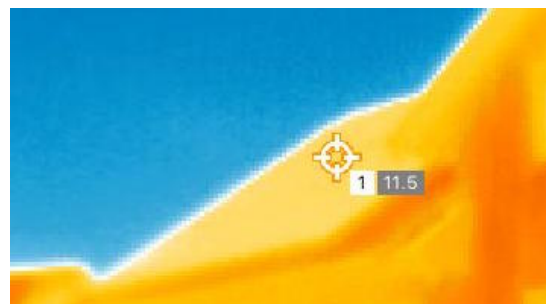
Figure C.7: Two thermal images of system 8, taken from different angles, indicating a constant temperature over the entire system. Note that the absolute temperatures shown in the images is wrong as temperature and emissivity references were not possible to set.
