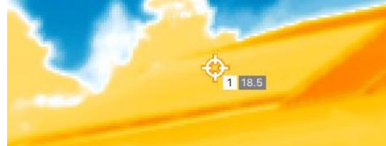
Figure C.8: Two thermal images of system 9, taken from different angles, indicating a constant temperature over the entire system. Note that the absolute temperatures shown in the images is wrong as temperature and emissivity references were not possible to set.
