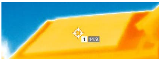
Figure C.7: Two thermal images of system 8, taken from different angles, indicating a constant temperature over the entire system. Note that the absolute temperatures shown in the images is wrong as temperature and emissivity references were not possible to set.
