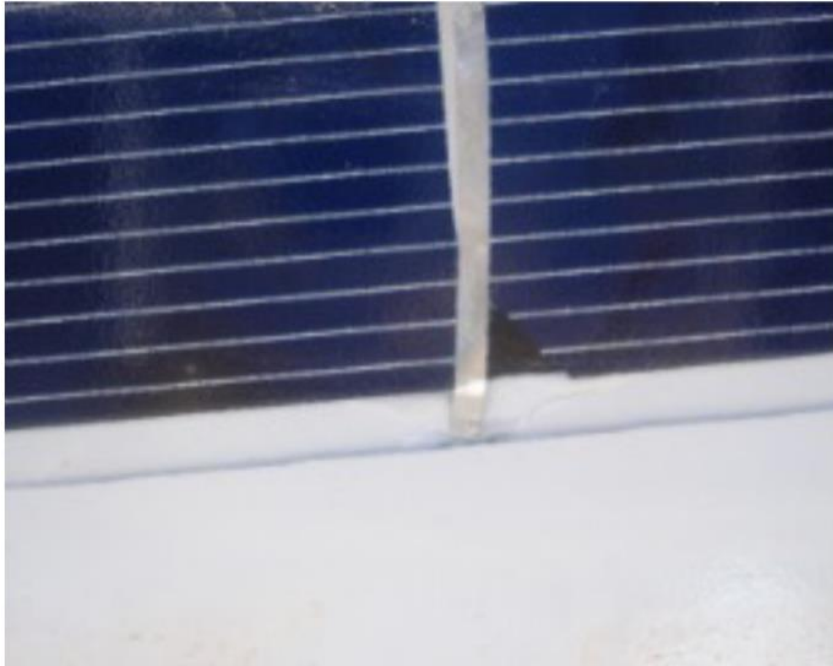
Figure 2.18 Illustration of a broken solar cell. Reused with permission (Díez-Mediavilla, et al., 2014)
