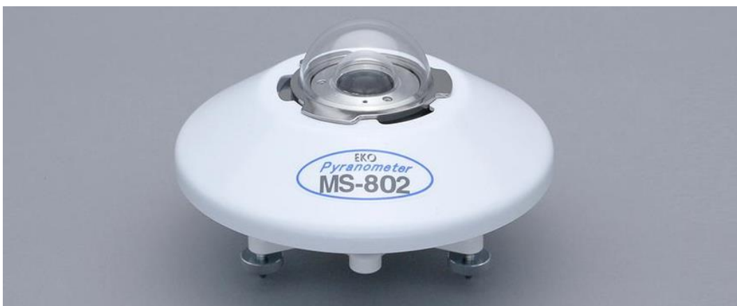
Figure 3.6 Picture of the MS802 pyranometer used at the site provided by EKO. The picture shows the black plate inside the two hemispherical domes of glass. In-between the two domes of glass there is a gas which reduces the conductivity, thus reducing the error in the measurements due to the environment temperature. Image copied by EKO with permission gained on 10.04.2019.
