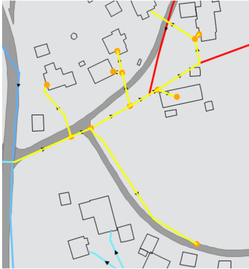
Figure 4-39: group of service connected to main branch-5
