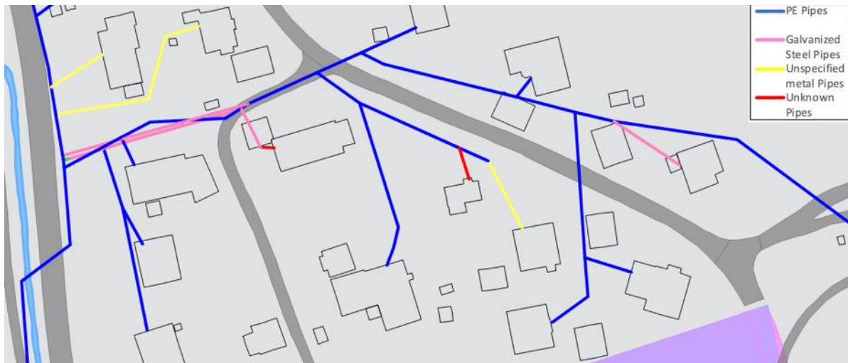
Figure 3-12: Predicting pipes' material-1
