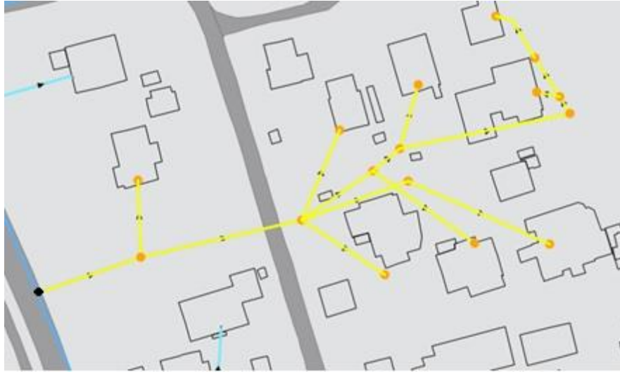
Figure 4-35: group of service connected to main branch-1
