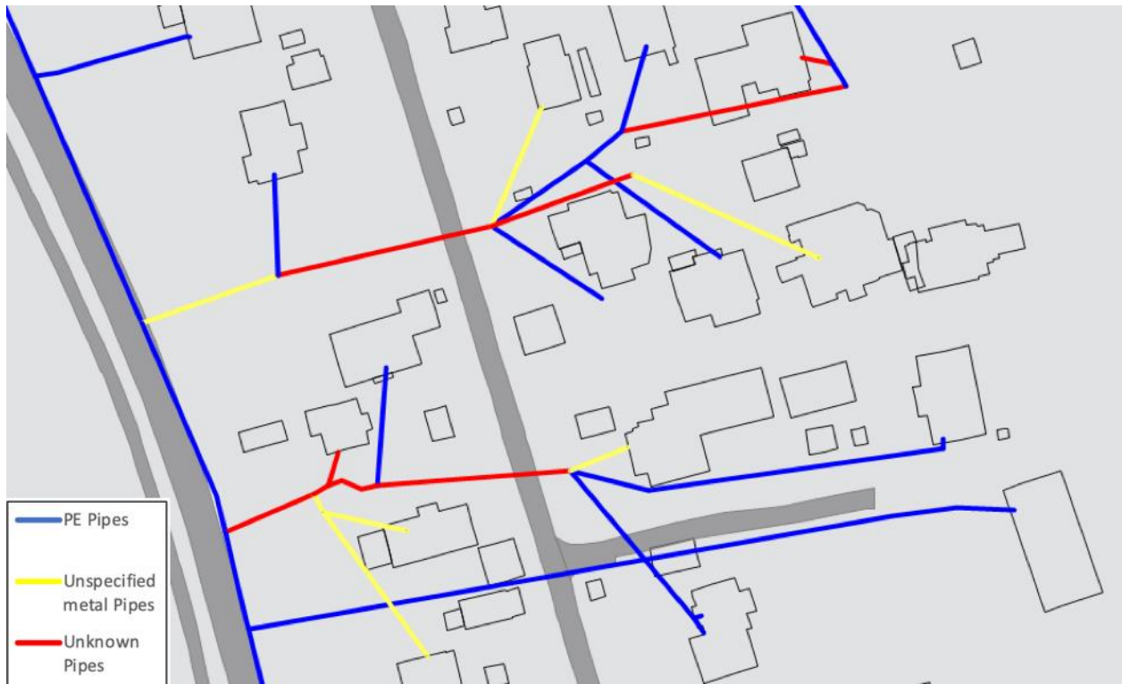
Figure 3-15: Predicting pipes' material-4
