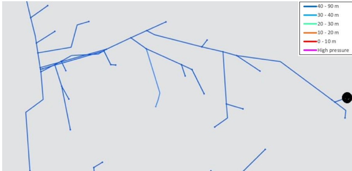
Figure 4-27: pressure result, for expected total water demand
