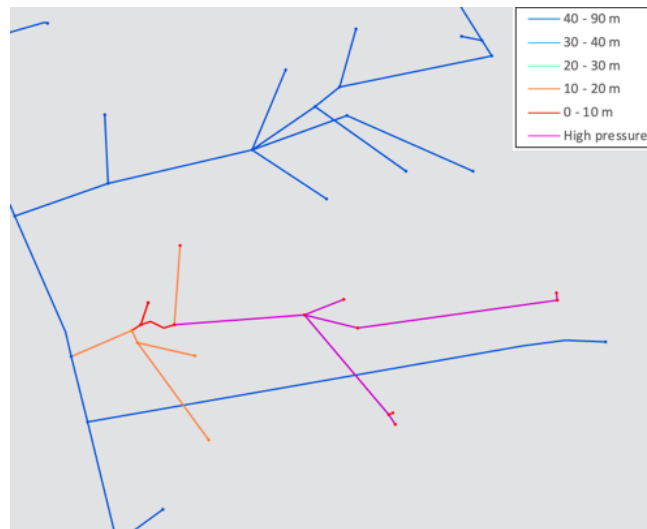
Figure 4-20: simulation results for expected total demand- Location 2
