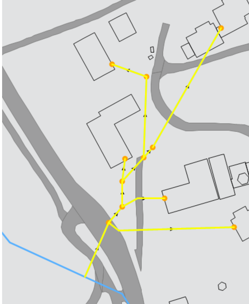
Figure 4-38: group of service connected to main branch-4
