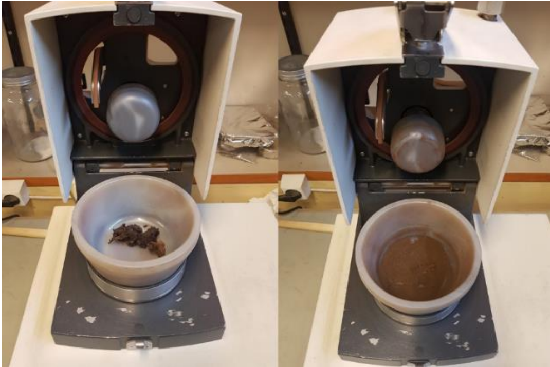
Figure 20: Picture of a peat sample before and after it was crushed in the mortar grinder. The samples were crushed in preparation of the total carbon and nitrogen analysis. Photo: Vera Sklet.
