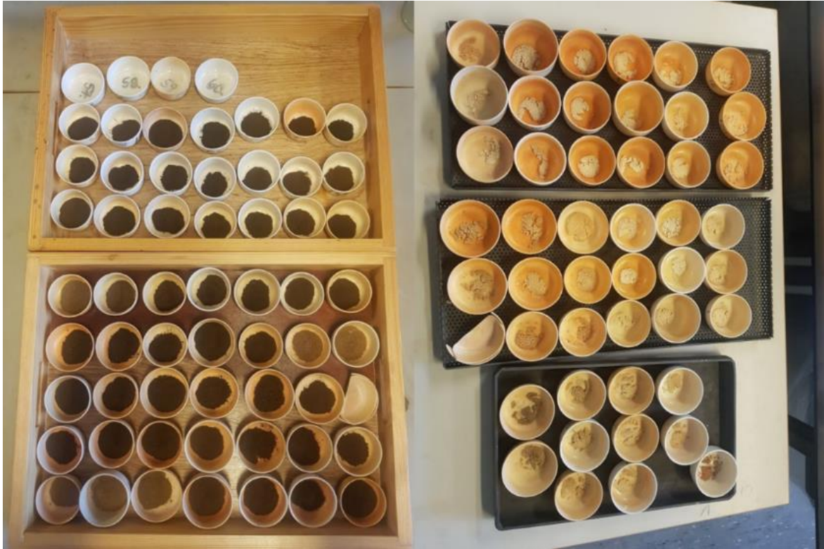
Figure 19: Photos of peat samples from core MM2 and MM3 before (left) and after (right) they were burned at 550 for the LOI test. Photos: Vera Sklet.
