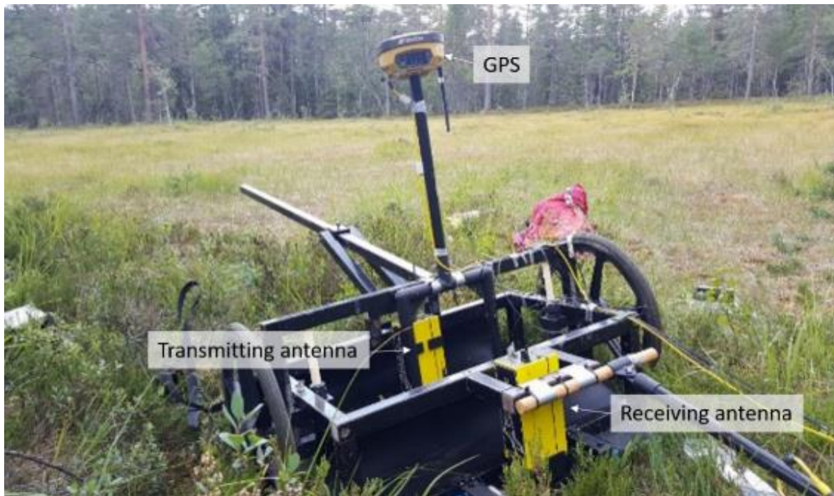
Figure 11: Setup of the GPR system used during fieldwork. The wheel that is used to measure the correct length of each profile is not showed in the picture. Photo: Per Holm Nygaard
