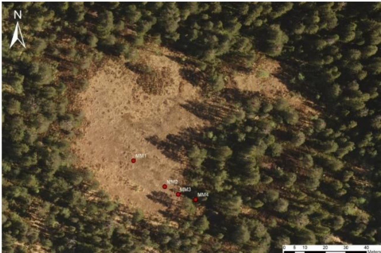
Figure 32: Placement of the four peat cores on Midtmyra is marked in red in this aerial photo. The location of core MM1 was chosen from where the deepest area was found from the GPR profiles. The location of the other three peat cores was chosen to find changes in soil properties in a transect from peat to forest soil. Modified from Kartverket (2019).
