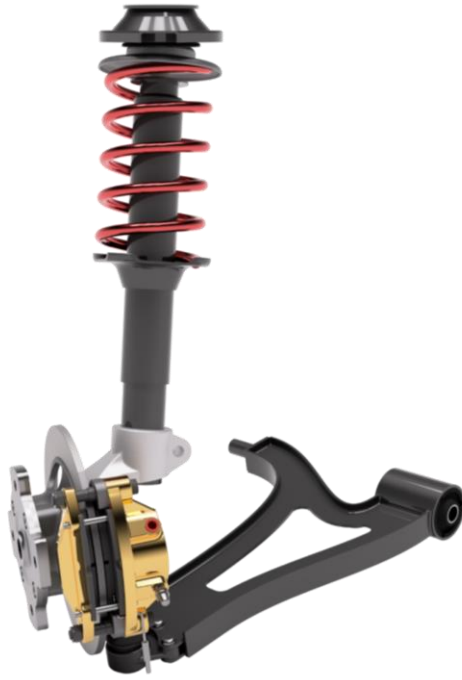
Figure 74. Wishbone shown in context, including purchased components.
