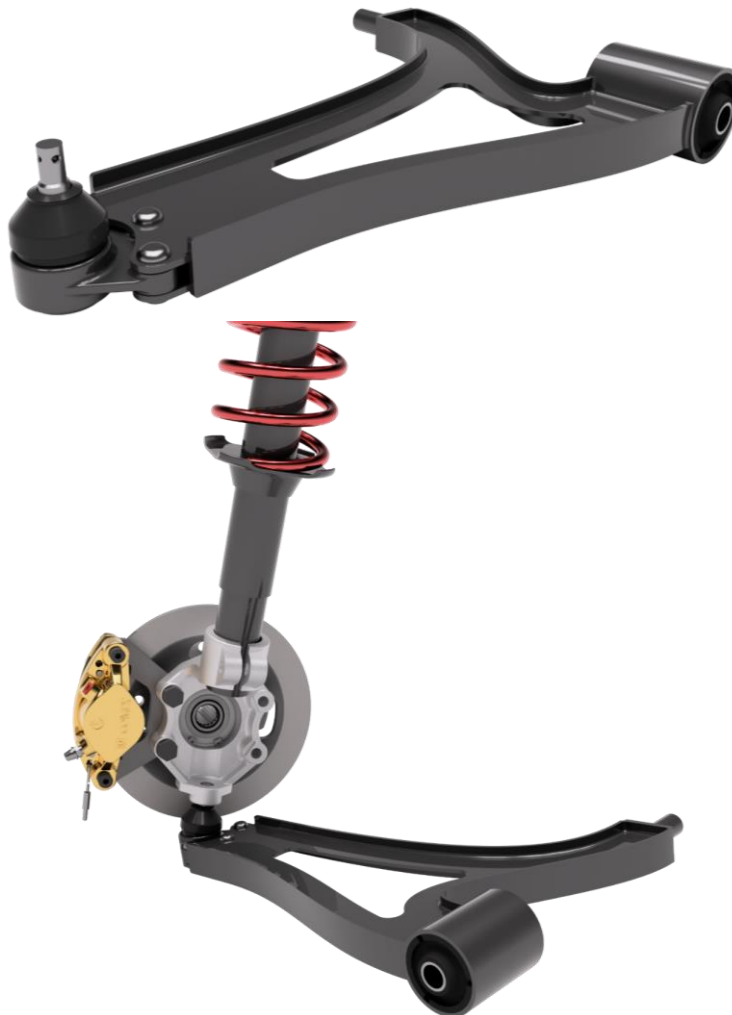
Figure 73. Wishbone shown in context, including purchased components.
