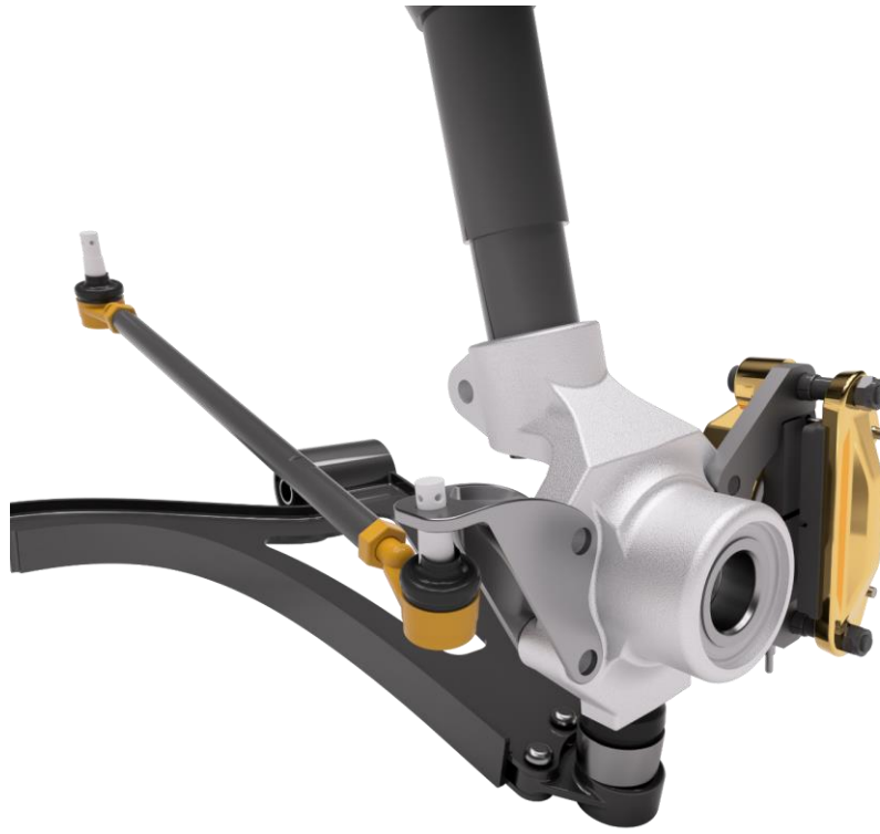
Figure 72 Steering bracket and wishbone shown in context, including purchased components.
