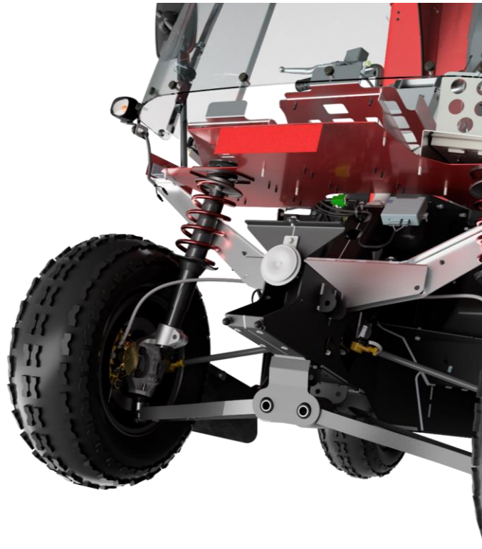
Figure 68. Location for wishbone and MacPherson Strut mounting.
