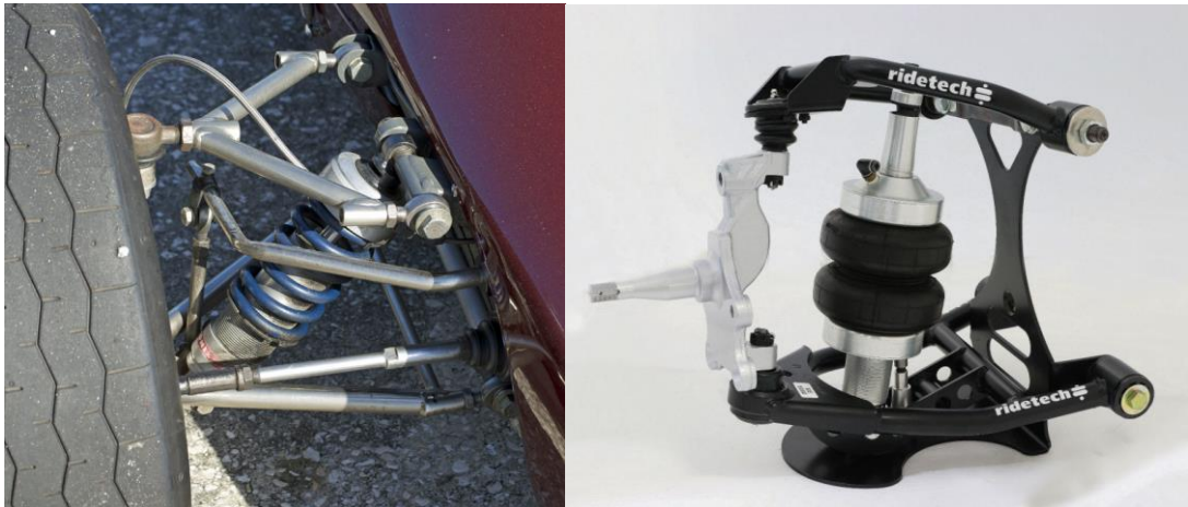
Figure 57. Double Wishbone utilizing Heim Joints (Left) and Double Wishbone utilizing bushings (Right) [43], [44].
