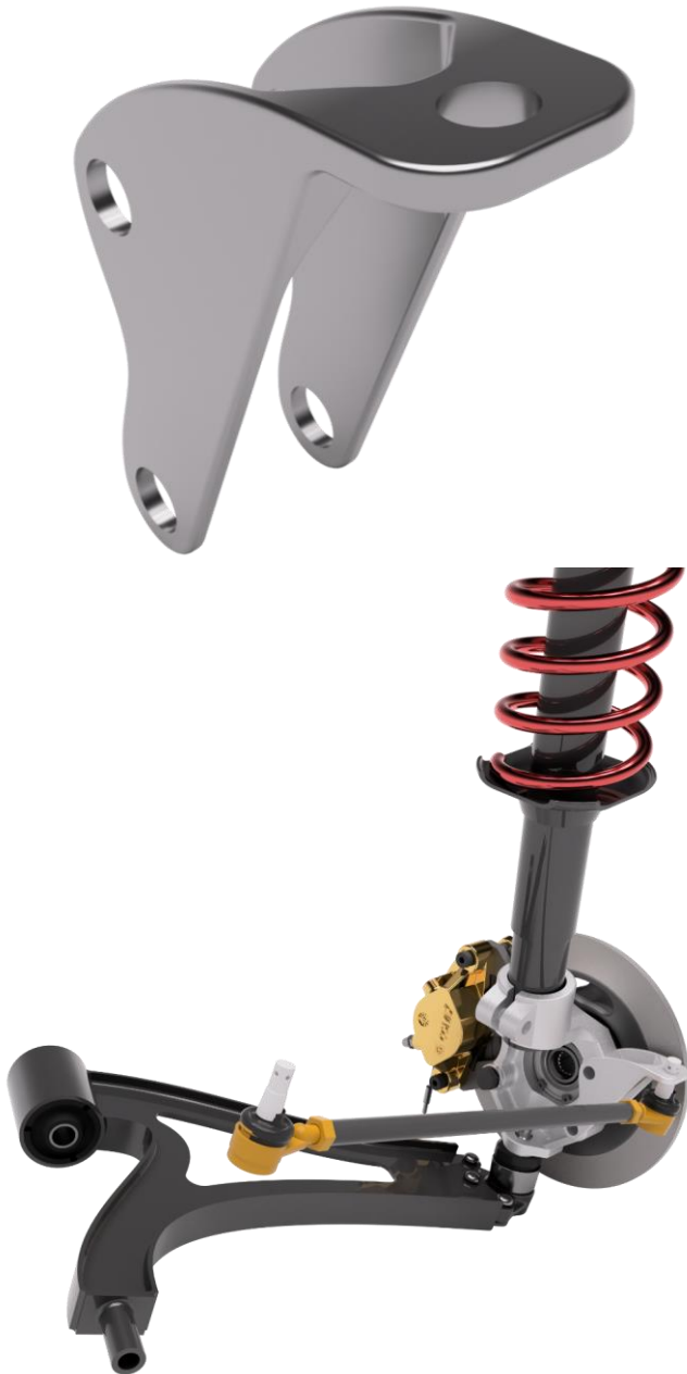
Figure 71. Steering bracket and wishbone shown in context, including purchased components.
