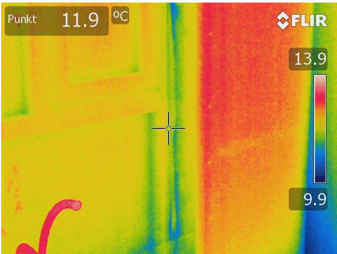
Kaldt felt langs vindusinnsetting
