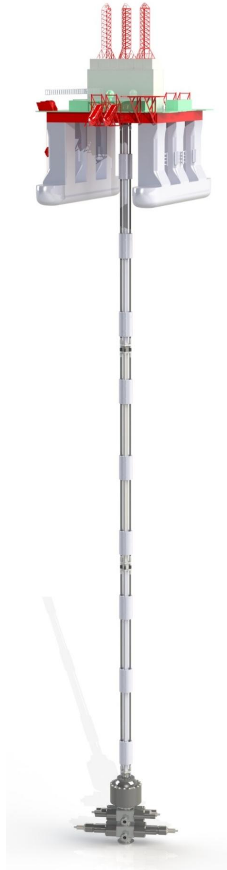
Figure 4 - Illustration of vessel, riser string and BOP.
