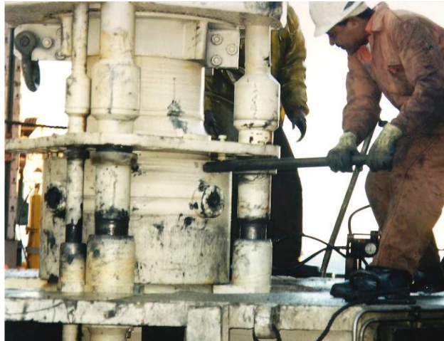
Figure 7 - The Lock ring is turned manually [17].
