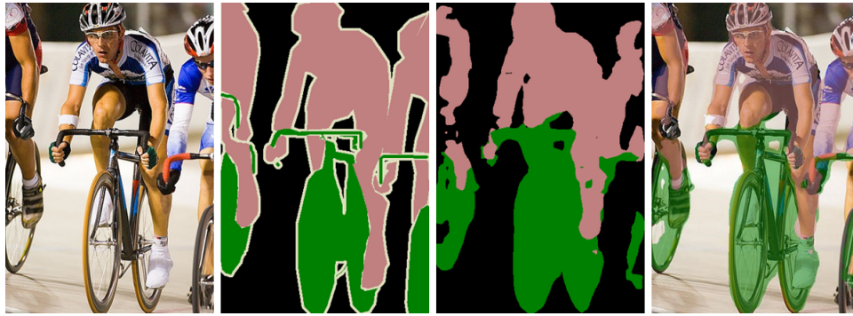
Figure 1.2: From the left: Input image, mask, predicted mask, input image overlaid with the predicted mask [32]
