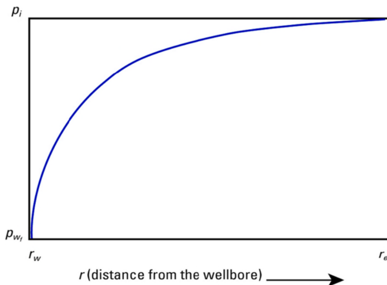
Figure 4.3: Pressure profile away from the wellbore (PetroWiki, n.d.-f).
