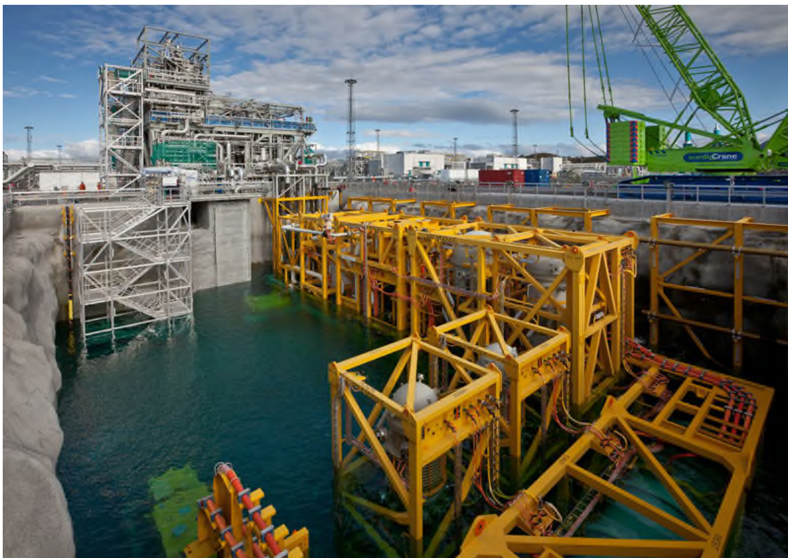
Figure 3.1: Ormen Lange Subsea Compression Pilot testing. Courtesy of Aker Solutions, Photo: Relevant Film AS
