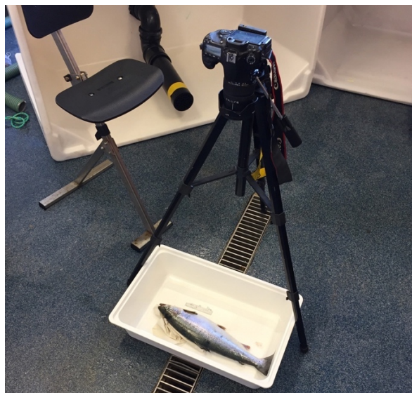
Figure 7 – The photoshoot setup during the third sampling session. A tripod was utilized in order to standardize the images. The white box made all the details of the fish much more visible.
