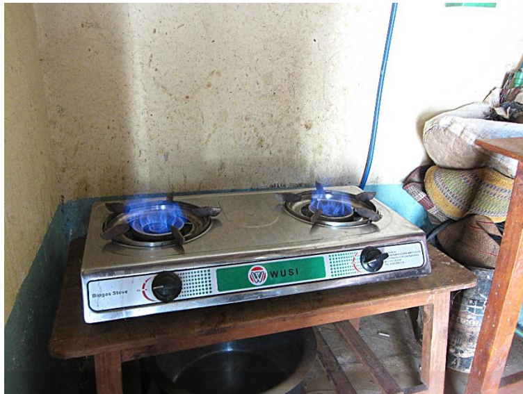
Figure 4: A biogas stove burning biogas. (Source: Heidi Hustad Gleditsch)
