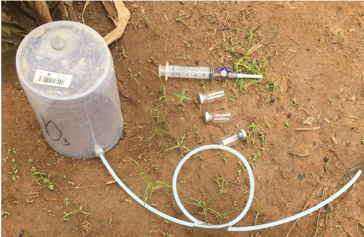
Image 1. Gas chamber (for \text{NO}_3 labeled plots) used for collecting gas samples along with syringes and vials used to obtain samples.
