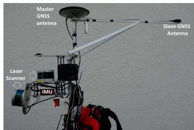
Figure 1. In-house-built backpack laser scanner.
