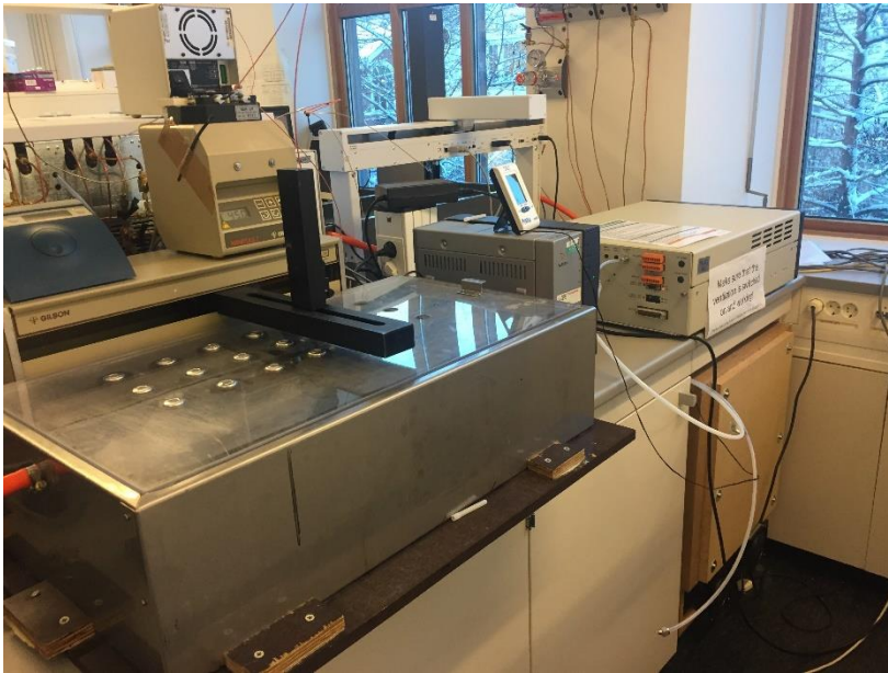
Figure 6: The robot set up. This is a picture of the old robot with only 15 stirring positions. There is a total of 3 robots today.
