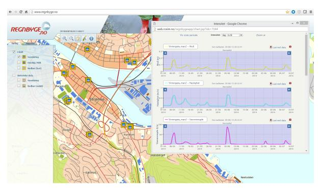
Fig. 2. The user interface of the regnbyge.no sewer surveillance system
