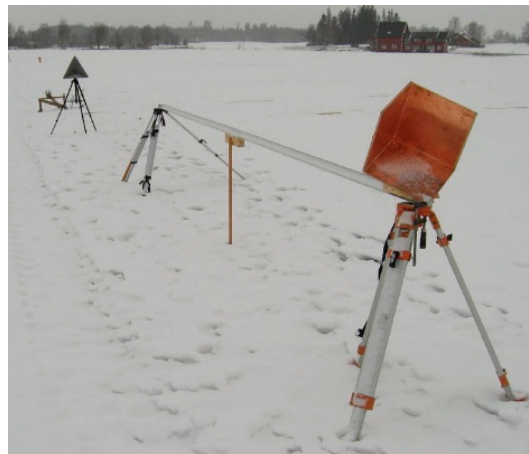
Figure 2. Picture showing the setup of the field experiment. The square trihedral corner reflector is in the front on top of the rail and in the rear is the reference triangular trihedral corner reflector on the tripod. Both the rail and the reference reflector were radially aligned to the look angle of the radar.
