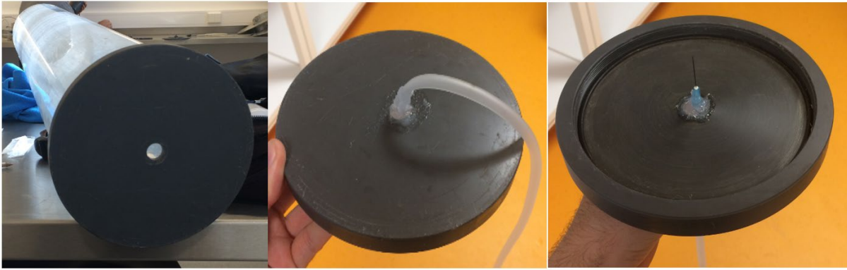
Figure 18. Hole through the PVC panel at the bottom of the tank (left), silicon tubing sealed and fed through the underside of the panel (centre), & needle extruding from the silicon tubing and sealant through the top side of the panel (right).
