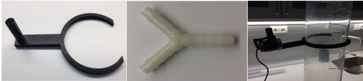
Figure 20. The webcam bracelet (left), airline splitter (centre) and webcam attached to the webcam bracelet (right).
