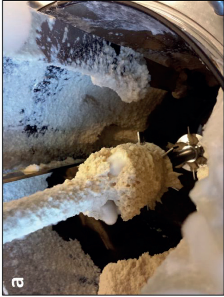
Fig. S5 Moritella alpina ATCC 32222 grown on impellers, baffles and wall of the 42 L total volume pre-pilot bioreactor. Aerial mycelium started to grow on baffles.
