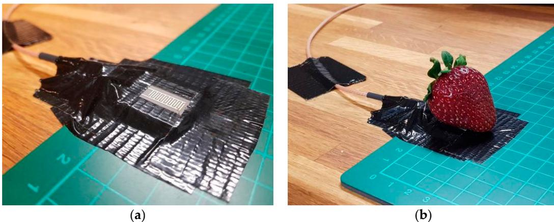
**Figure 3.** (a) 8-pair IDE sensor, with only sensitive element exposed and (b) example with fruit in place for measurement.
