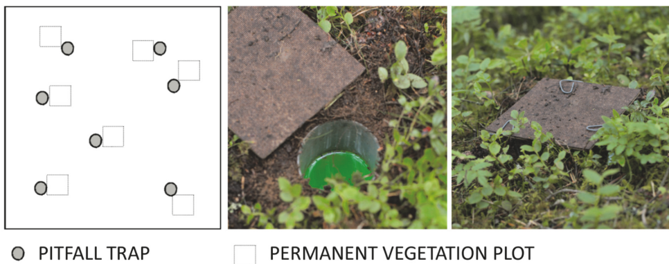
Figure 6. Illustration of pitfall traps in the macroplot (left). We collected ground-dwelling beetles with seven pitfall traps in each macroplot, placed adjacent to each permanent vegetation plot (middle). We protected each trap with a wooden roof, about 5–10 cm above the trap, to prevent litter to fall in, or rain to flood the trap (right). Photo: Lilleeng, M. S.
