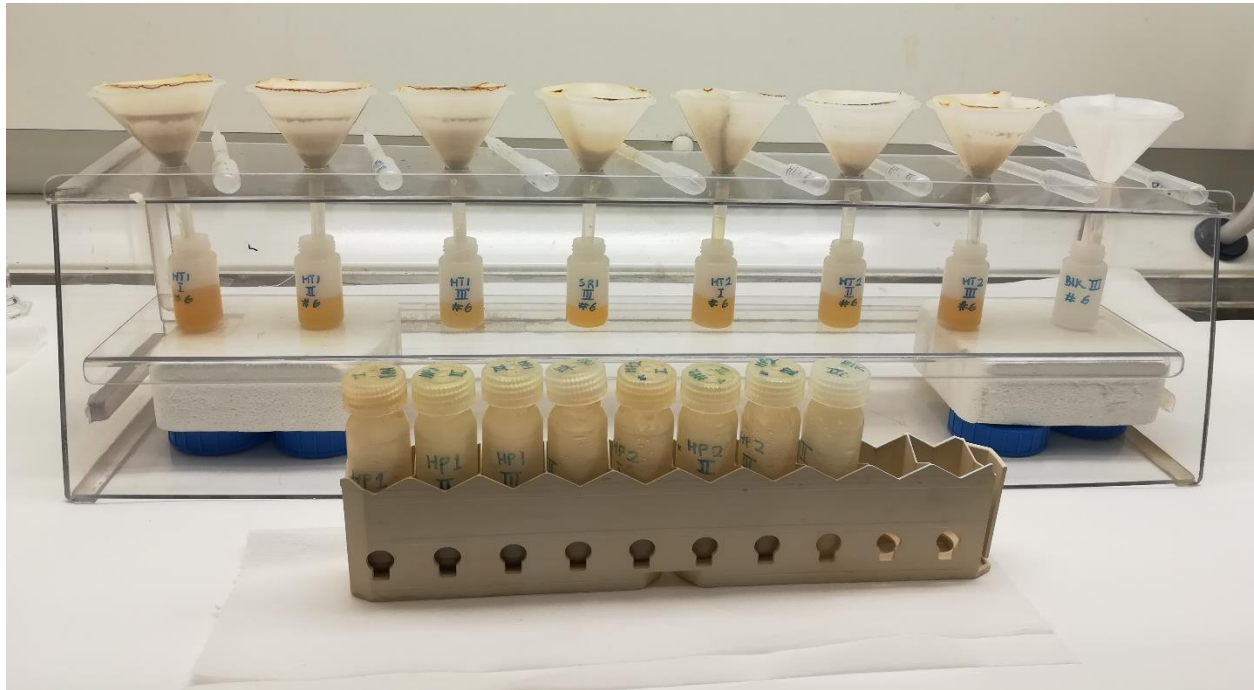
Figure 7: Experimental setup for the sequential extraction; plastic pipette beside funnels with inserted filters, placed in a funnel holder over sample vials, and centrifuge tubes in a rack.
