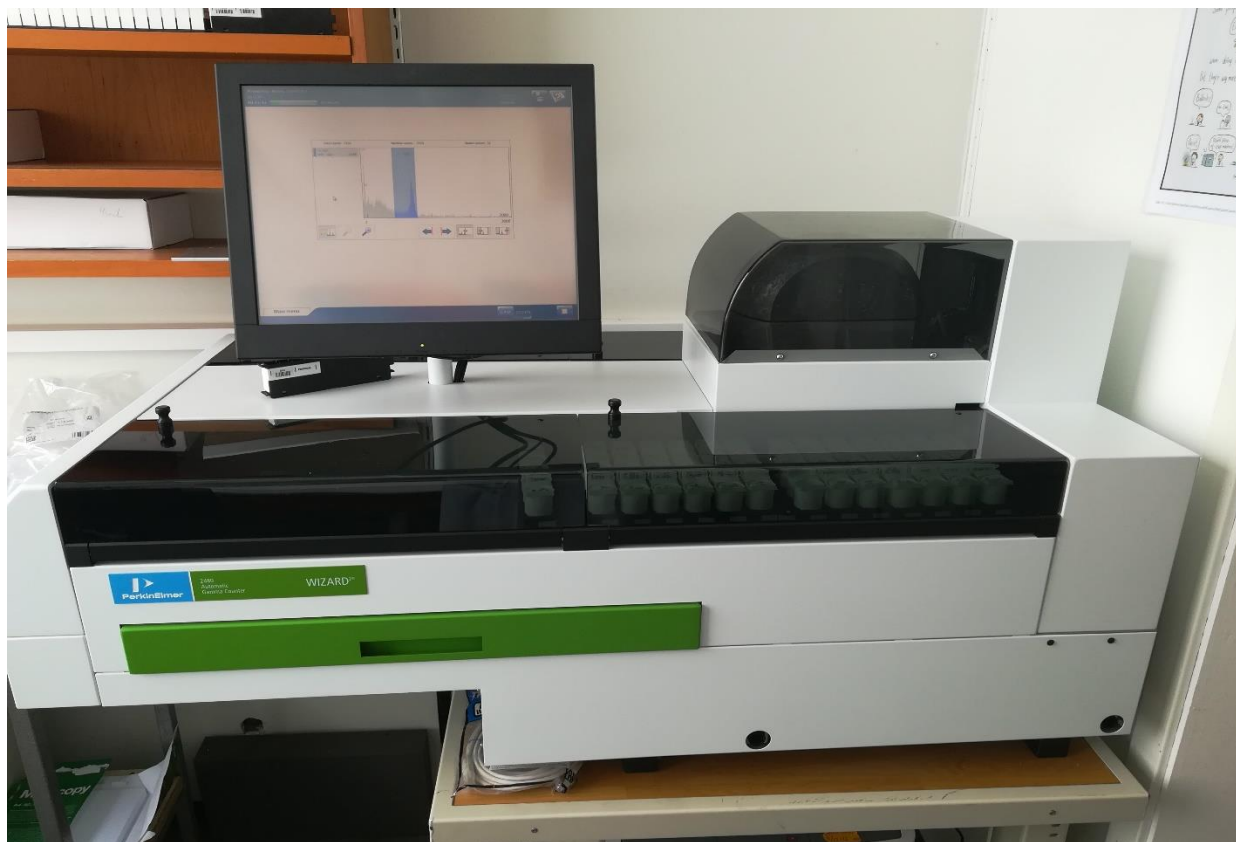
Figure 8: Gamma measurements on NaI detector (PerkinElmer Wizard2® 2480 Automatic Gamma Counter)
