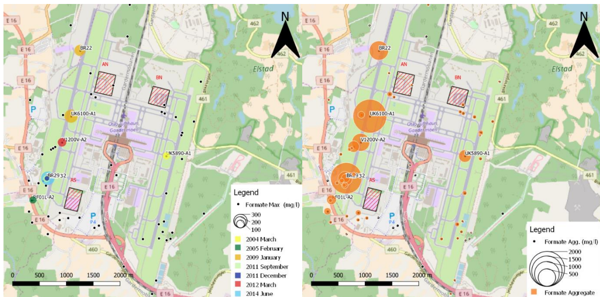
Figure 4.14 – Left: Maximum values of Pfo measured; Right: Accumulative of all the measurements taken at each monitoring well since year 2001.
