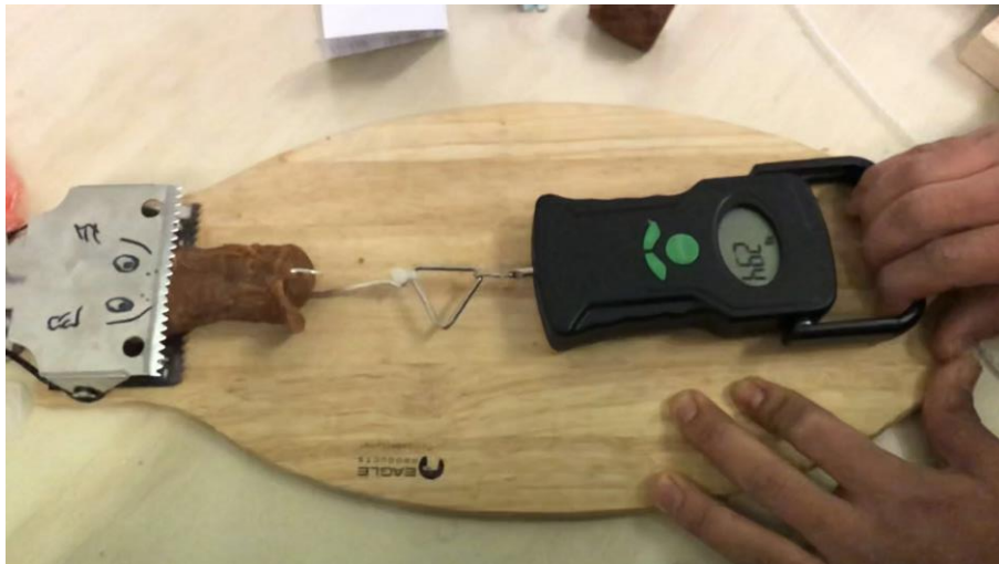
Figure 12. Measuring the tensile strength of the sample.
