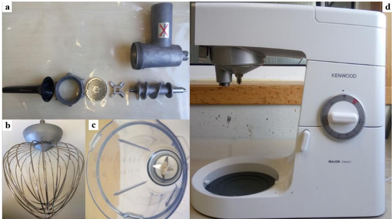
Figure 7. (a) Mincing elements; (b) blender; (c) grinder; (d) mincing and grinding device
