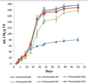
**Fig. 1** Cumulative methane production reactors fed with untreated birch without bioaugmentation (closed triangles), steam-exploded birch without bioaugmentation (open triangles, as well as steam-exploded birch with applied bioaugmentation at different *C. bescii* loadings (2% v/v open circles; 5% v/v crosses; 10% v/v open squares; and 15% v/v closed circles)
