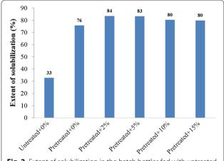
**Fig. 2** Extent of solubilization in the batch bottles fed with untreated birch without bioaugmentation, steam-exploded birch without bioaugmentation and steam-exploded birch with applied bioaugmentation at different *C. bescii* loadings from 2 to 15% v/v
