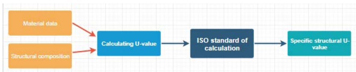
Figure 2- The methodical approach used to calculate U-value, according to ISO standard 6946:2014.
