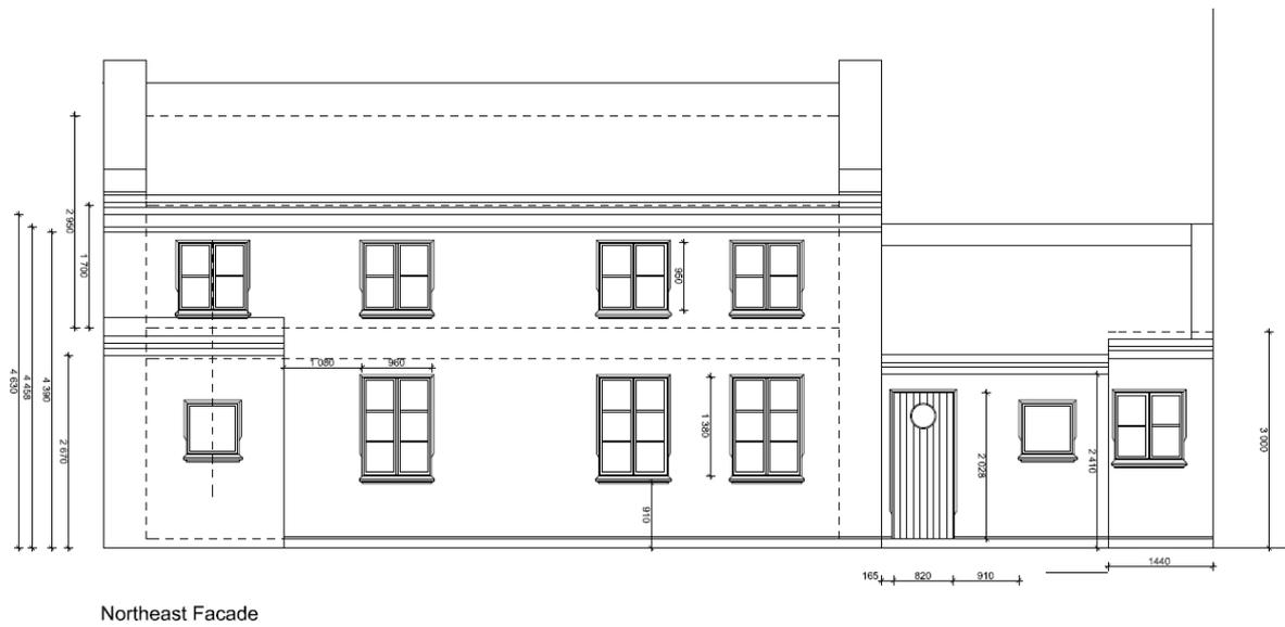
Figure 25-Blueprint of the Northeast façade of Bergsliens Gate 12B-C. (Source: Boligbygg).
