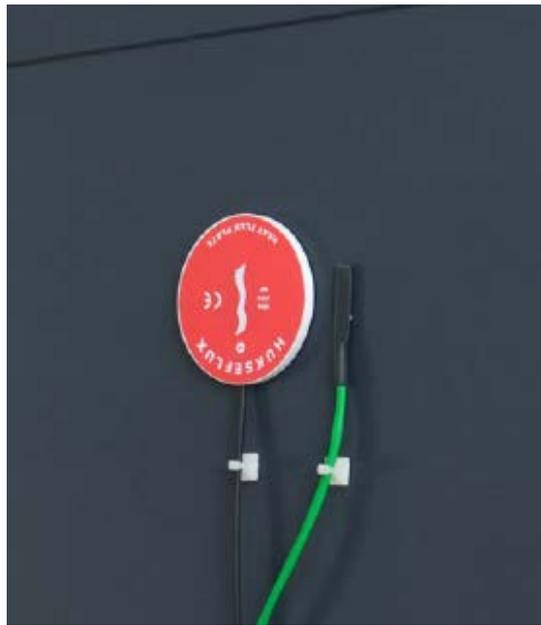
Figure 33- Heat flux sensor and temperature sensor (warm side)
