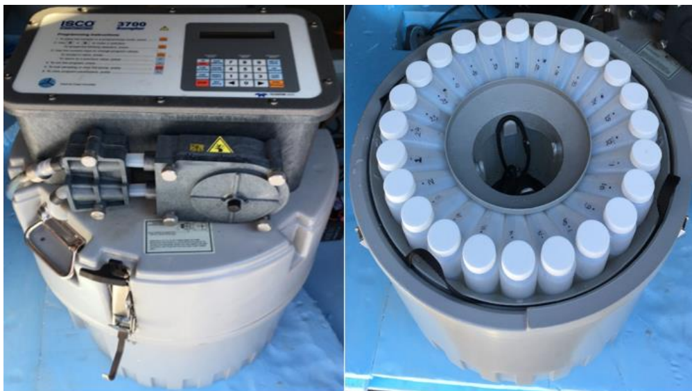
Figure 5 ISCO 3700 portable auto sampler at the sampling point, Våkas.
