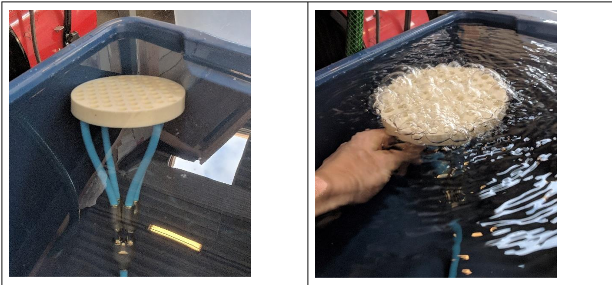
Figure 7.2-1 A) Diffuser submerged with splitters B) Diffuser tested underwater with compressor.
