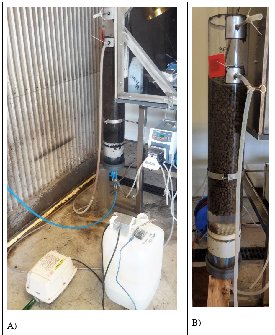
Figure 7.3-1 A) Overview of biofilter system in operation with biomedica with grown biofilm B) Column in test phase with biomedica without biofilm.
