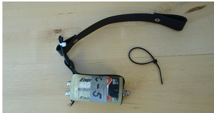
Figure 4: Example of a dummy telemetry-collar used in the study. The collars consisted of a BioThane® strap and affixed epoxy moulded C battery. The cable tie was used as a lock.
