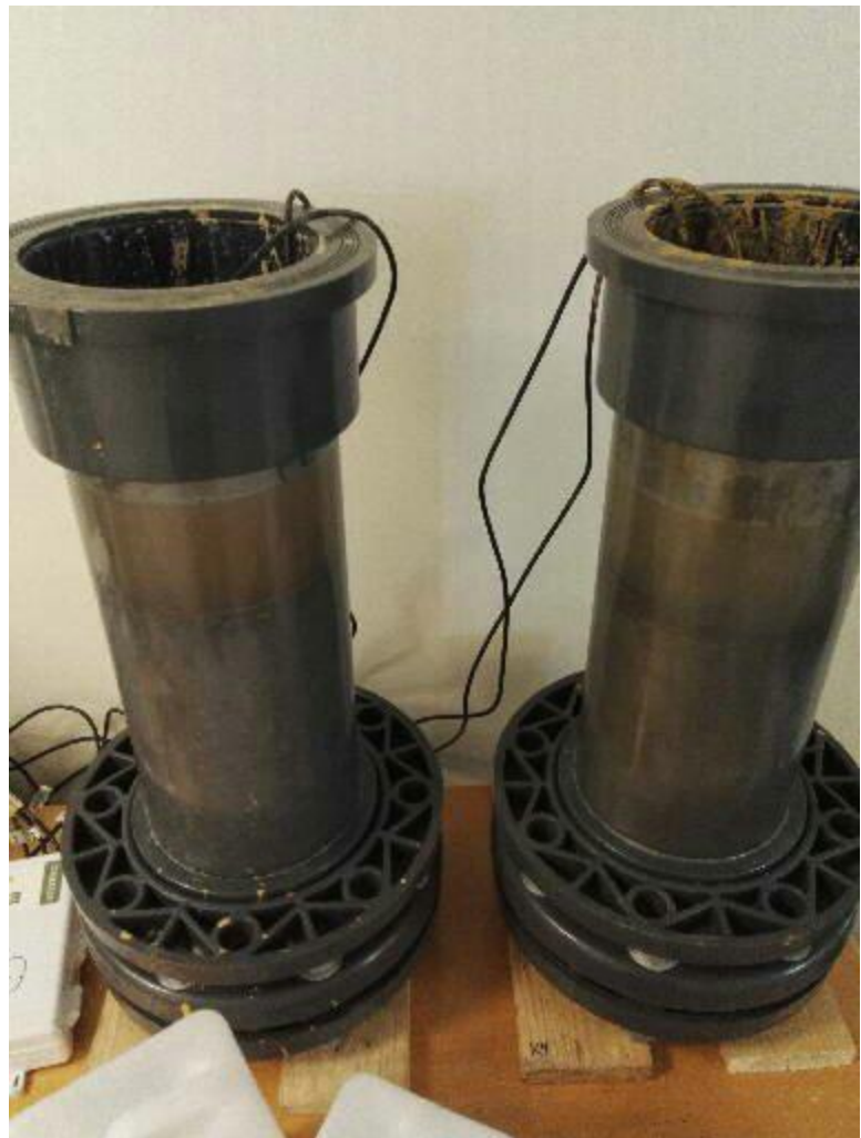
Fig 4.3 Picture of large columns: the left column is filled with reactive tailings (Source Tvedten, 2016)
