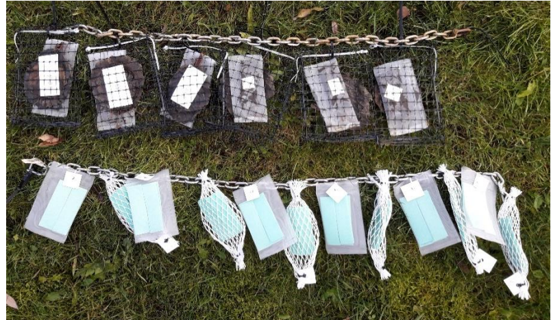
Figure 4: Photograph of setup for litter decay experiment: On top is the leaf litter with the small meshed bags inside the large meshed bags, and on bottom is the Wettex sponge cloth with the small and large meshed bags alternating down the chain.
